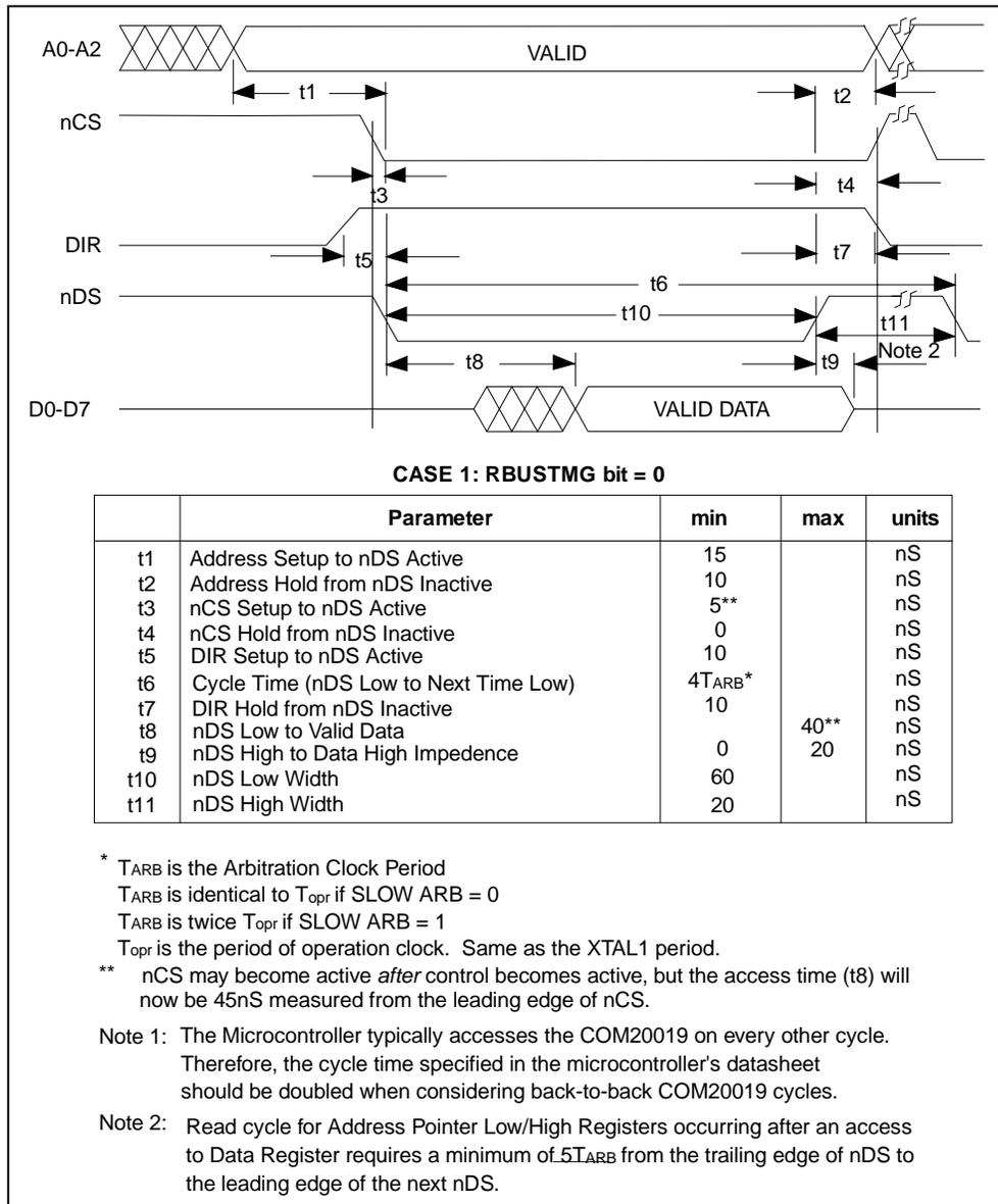
**Figure 8.7 - NON-MULTIPLEXED BUS, 68XX-LIKE CONTROL SIGNALS; READ CYCLE**
