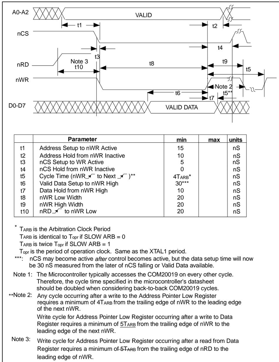
**Figure 8.9 - NON-MULTIPLEXED BUS, 80XX-LIKE CONTROL SIGNALS; WRITE CYCLE**
