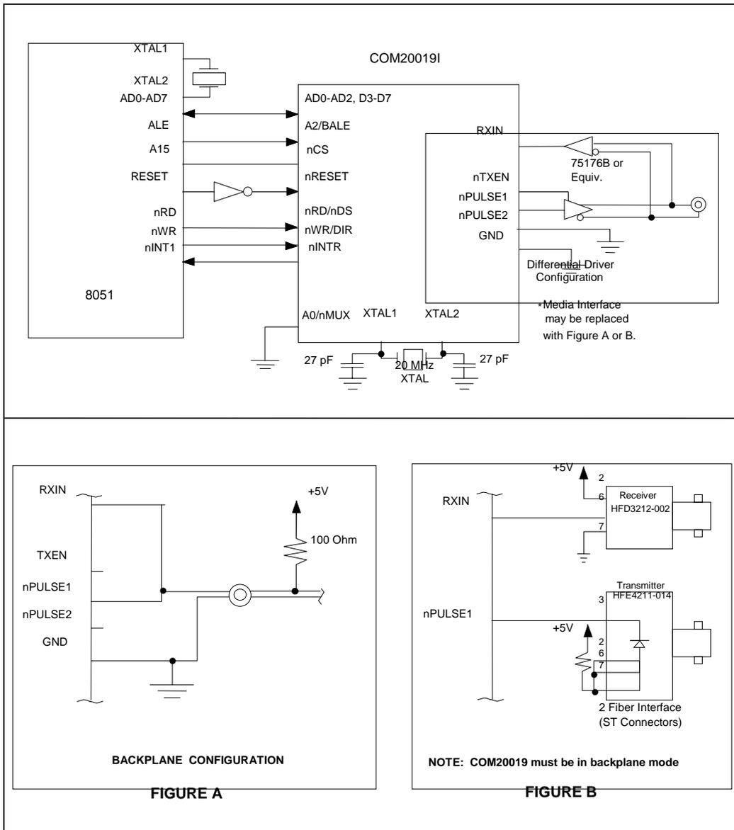
**Figure 5.1 - MULTIPLEXED, 8051-LIKE BUS INTERFACE WITH RS-485 INTERFACE**
