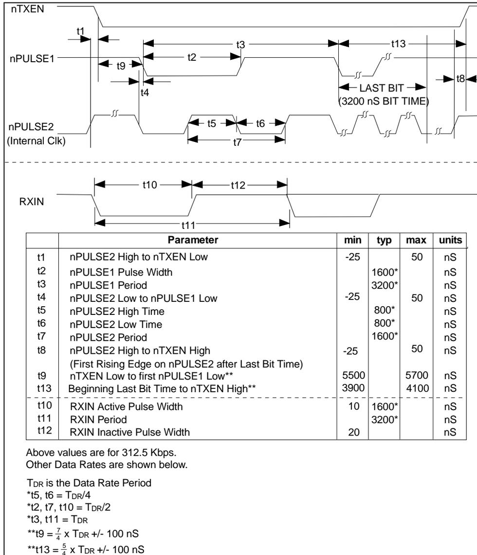
**Figure 8.11 - BACKPLANE MODE TRANSMIT OR RECEIVE TIMING**
