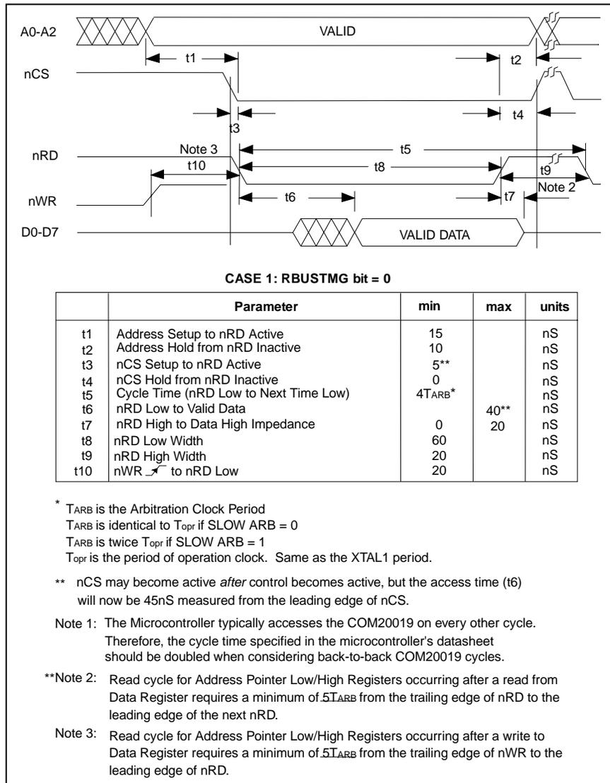
**Figure 8.5 - NON-MULTIPLEXED BUS, 80XX-LIKE CONTROL SIGNALS; READ CYCLE**
