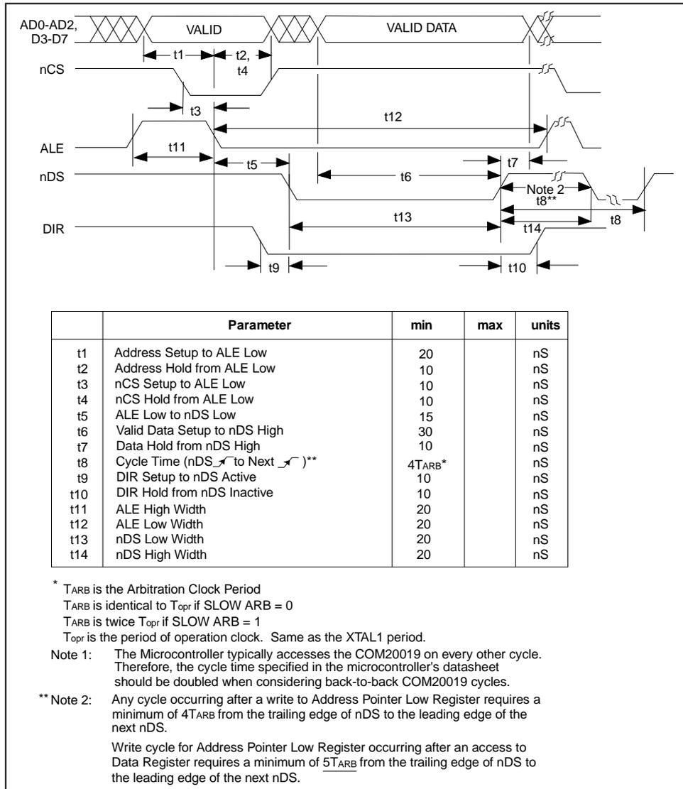
**Figure 8.3 - MULTIPLEXED BUS, 68XX-LIKE CONTROL SIGNALS; WRITE CYCLE**
