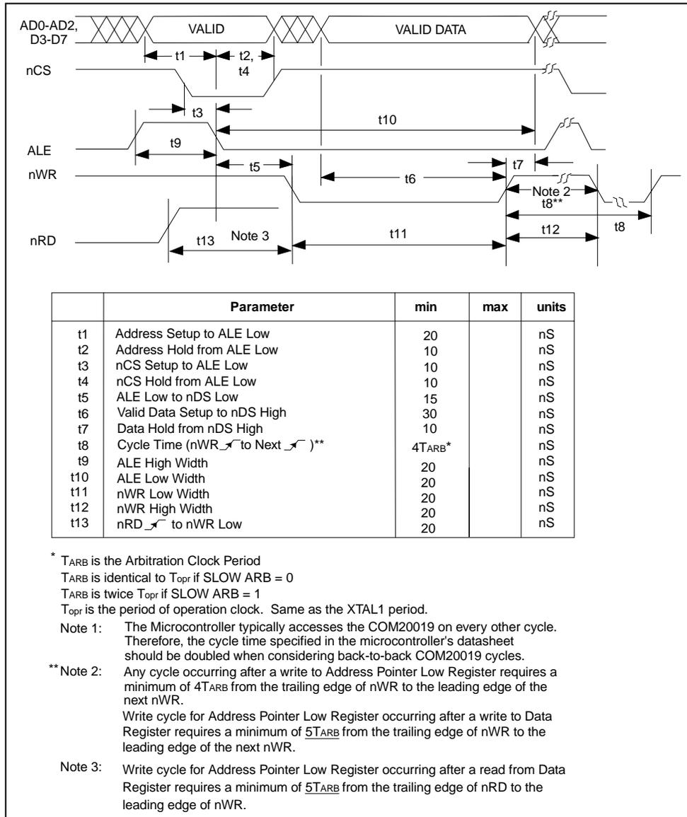
Figure 8.4 - MULTIPLEXED BUS, 80XX-LIKE CONTROL SIGNALS; WRITE CYCLE
