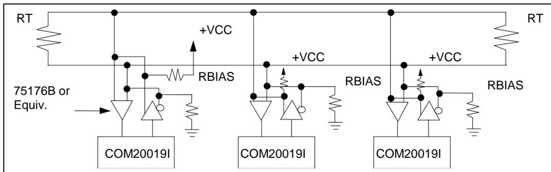
**Figure 5.4 - COM20019I NETWORK USING RS-485 DIFFERENTIAL TRANSCIEVERS**
