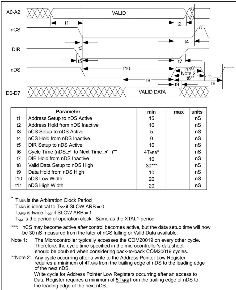
Figure 8.10 - NON-MULTIPLEXED BUS, 68XX-LIKE CONTROL SIGNALS; WRITE CYCLE
