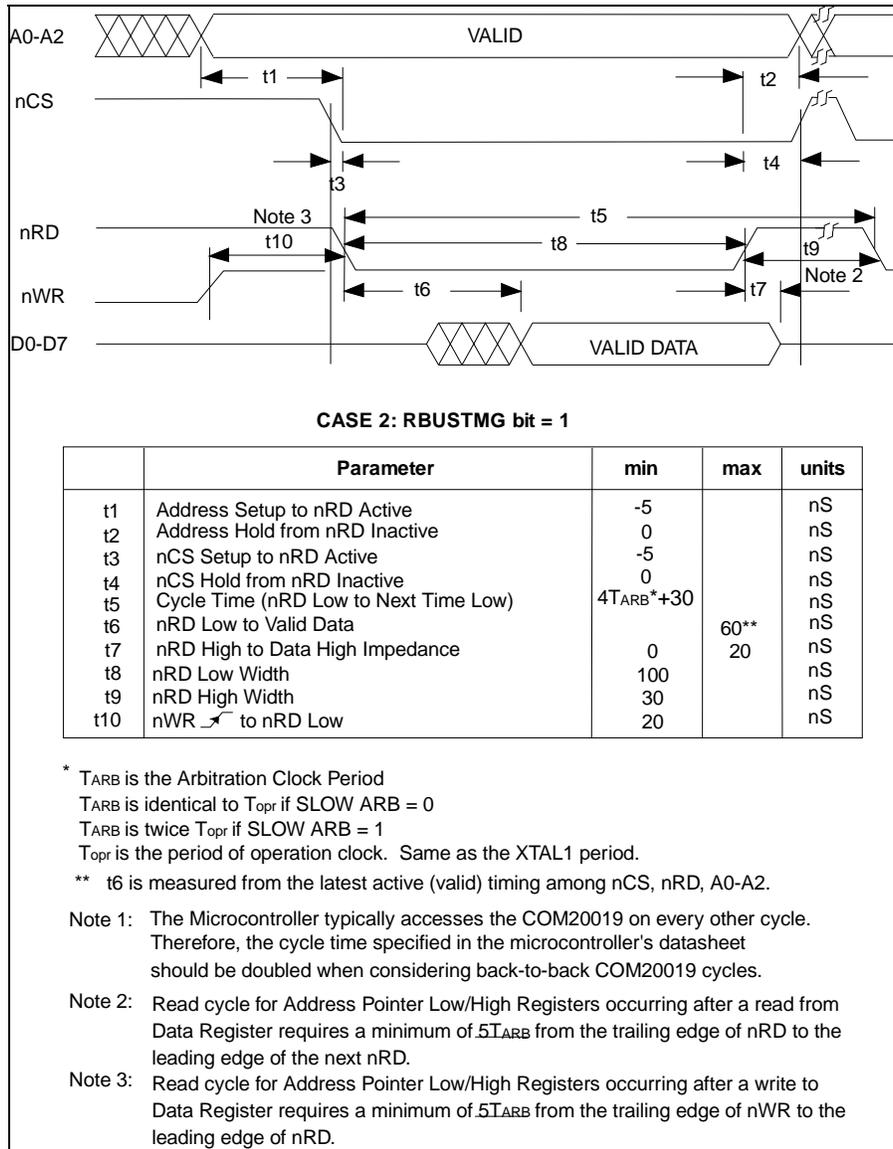
**Figure 8.6 - NON-MULTIPLEXED BUS, 80XX-LIKE CONTROL SIGNALS; READ CYCLE**
