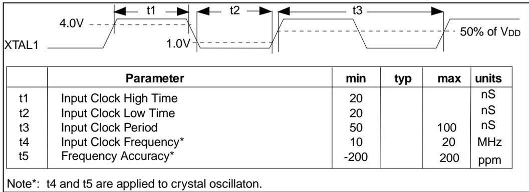
Figure 8.12 - TTL INPUT TIMING ON XTAL1 PIN
