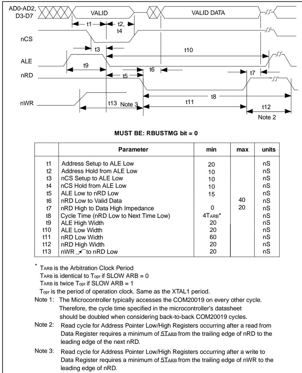
**Figure 8.2 - MULTIPLEXED BUS, 80XX-LIKE CONTROL SIGNALS; READ CYCLE**
