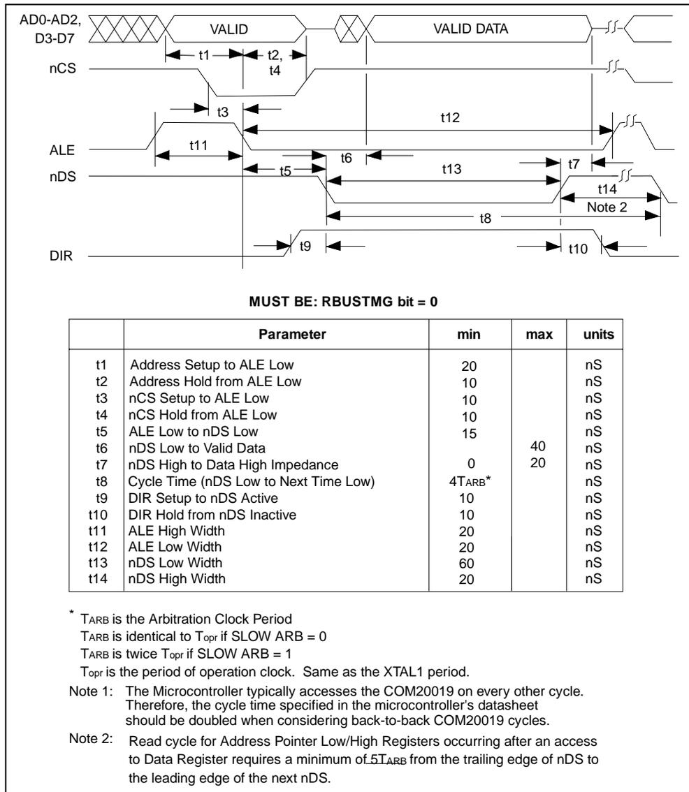
Figure 8.1 - MULTIPLEXED BUS, 68XX-LIKE CONTROL SIGNALS; READ CYCLE
