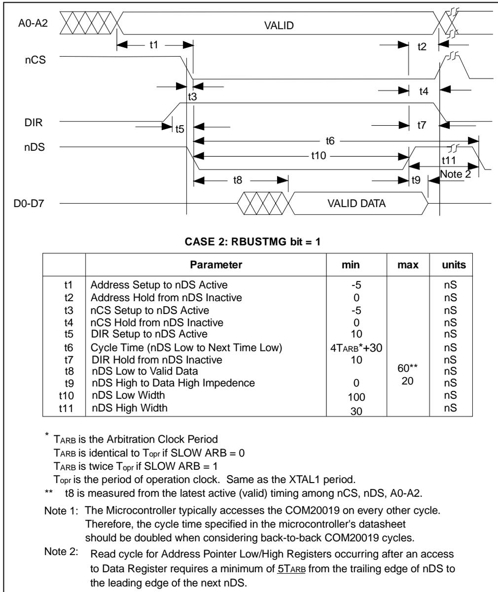
**Figure 8.8 - NON-MULTIPLEXED BUS, 68XX-LIKE CONTROL SIGNALS; READ CYCLE**
