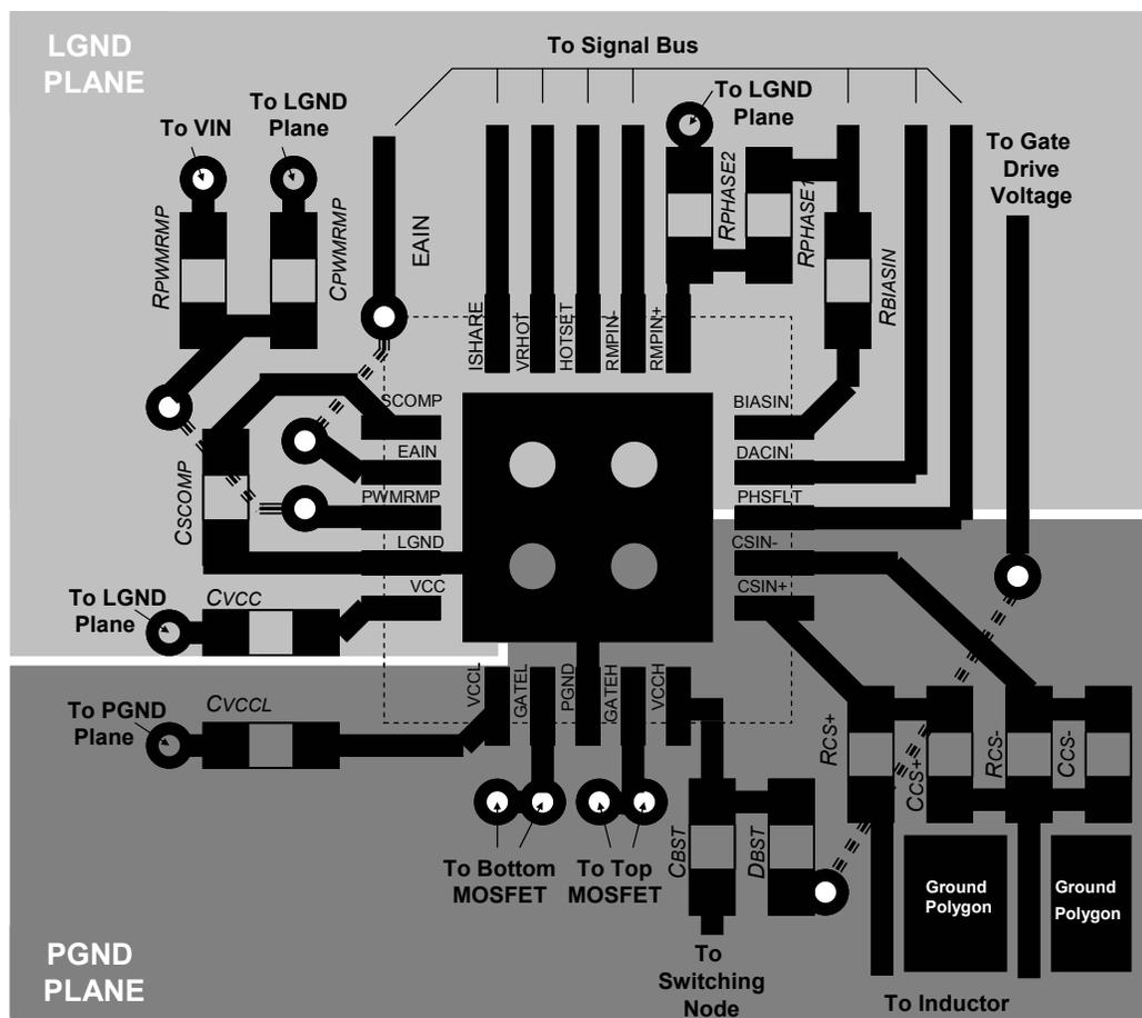
**PCB Metal and Component Placement**
