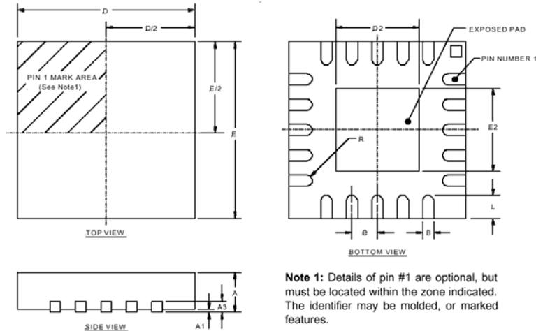
**Note 1:** Details of pin #1 are optional, but must be located within the zone indicated. The identifier may be molded, or marked features.
