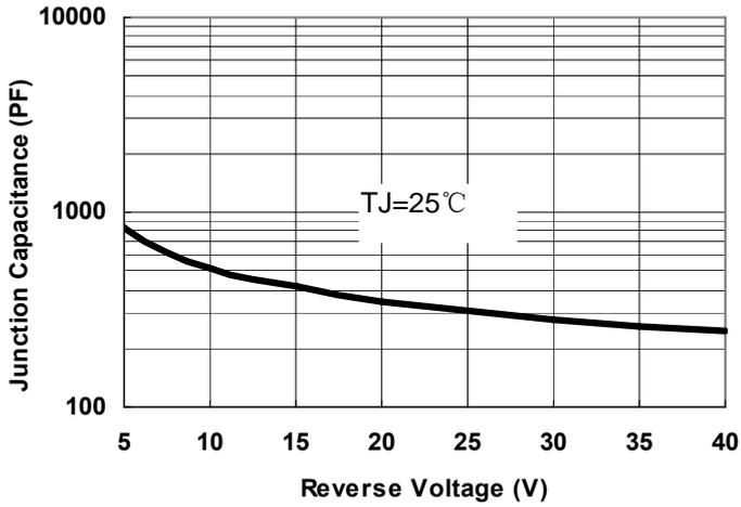
**Fig.1-Typical Junction Capacitance**
