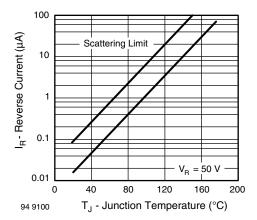
Fig. 1 - Reverse Current vs. Junction Temperature
