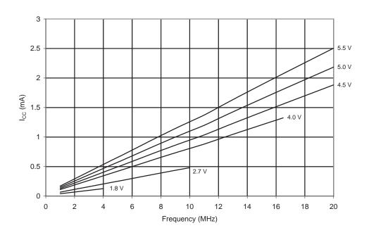
$\textbf{Figure 20-8.} \hspace{0.5cm} \textbf{Idle Supply Current vs. } V_{\text{CC}} \hspace{0.1cm} \textbf{(Internal Calibrated Oscillator, 8 MHz)}$
