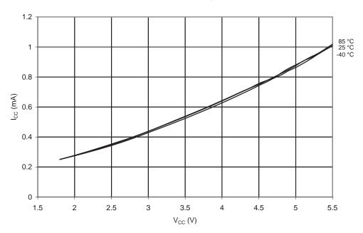
Figure 20-5. Active Supply Current vs. V<sub>CC</sub> (Internal Calibrated Oscillator, 128 kHz)
