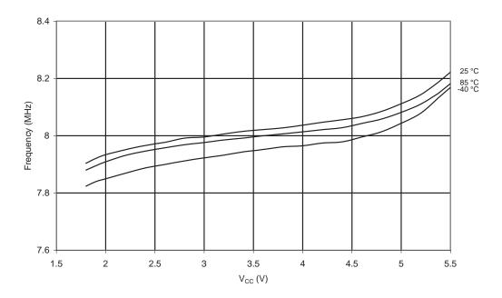
Figure 20-101. Frequency of Calibrated 8.0 MHz Oscillator vs. Temperature
