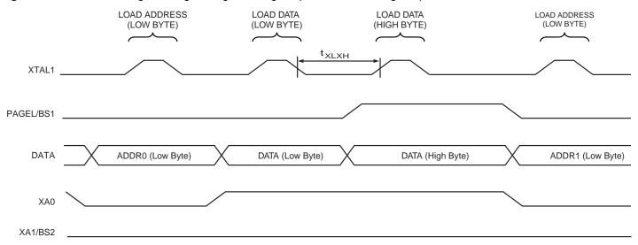
Note: The timing requirements shown in Figure 19-5 (i.e.,  $t_{DVXH}$ ,  $t_{XHXL}$ , and  $t_{XLDX}$ ) also apply to loading operation.
