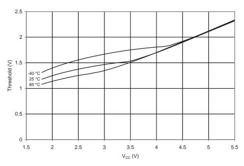
Figure 20-142.  $V_{IL}$ : Input Threshold Voltage vs.  $V_{CC}$  (Reset Pin, Read as '0') RESET INPUT THRESHOLD VOLTAGE vs. VCC  $V_{IL}$ . PIN READ AS '0'
