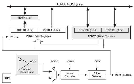
Figure 11-4. Input Capture Unit Block Diagram
