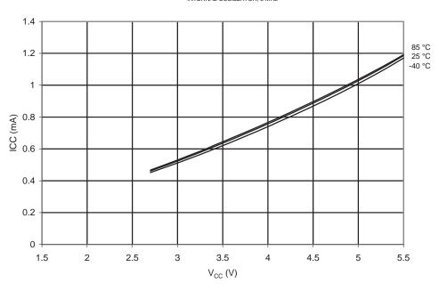
$\textbf{Figure 20-9.} \hspace{0.5cm} \textbf{Idle Supply Current vs. } V_{\text{CC}} \hspace{0.1cm} \textbf{(Internal Calibrated Oscillator, 1 MHz)}$
