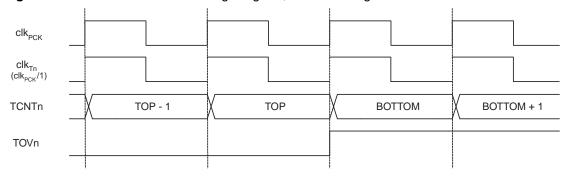
Figure 12-16 shows the same timing data, but with the prescaler enabled, in all modes other than Phase and Frequency Correct PWM Mode.
