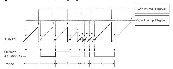
The counter value (TCNT1) that is shown as a histogram in Figure 12-11 is incremented until the counter value matches the TOP value. The counter is then cleared at the following clock cycle The diagram includes the Waveform Output (OCW1x) in toggle Compare Mode. The small horizontal line marks on the TCNT1 slopes represent Compare Matches between OCR1x and TCNT1.
