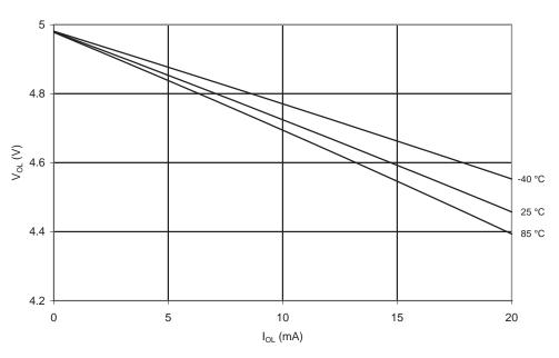
Figure 20-134.  $V_{OL}$ : Output Voltage vs. Sink Current (Reset Pin as I/O,  $V_{CC}$  = 5V)
