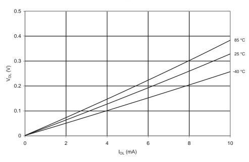
Figure 20-28.  $V_{OL}$ : Output Voltage vs. Sink Current (I/O Pin,  $V_{CC} = 5V$ )
