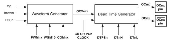
The tasks are shared as follows: the Waveform Generator generates the output (OCW1x) and the Dead Time Generator generates the non-overlapping PWM output pair from the output. Three Dead Time Generators are provided, one for each PWM output. The non-overlap time is adjustable and the PWM output and it's complementary output are adjusted separately, and independently for both PWM outputs.
