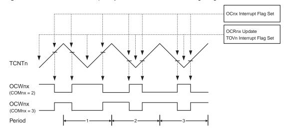
The Timer/Counter Overflow Flag (TOV1) is set each time the counter reaches BOTTOM. The Interrupt Flag can be used to generate an interrupt each time the counter reaches the BOTTOM value.
