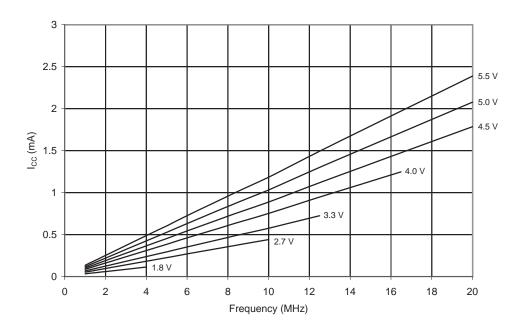
Figure 20-110. Idle Supply Current vs.  $V_{\text{CC}}$  (Internal Calibrated Oscillator, 8 MHz)
