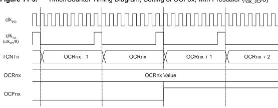
Figure 11-9. Timer/Counter Timing Diagram, Setting of OCF0x, with Prescaler (f<sub>clk I/O</sub>/8)
