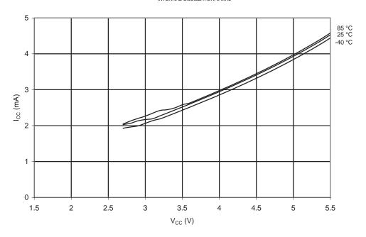
$\textbf{Figure 20-55.} \quad \text{Active Supply Current vs. V}_{\text{CC}} \text{ (Internal Calibrated Oscillator, 1 MHz)}$
