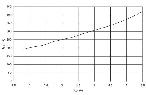
Figure 20-17. Timer/Counter1 Current vs. V<sub>CC</sub>
