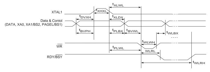
Figure 19-6. Parallel Programming Timing, Loading Sequence with Timing Requirements
