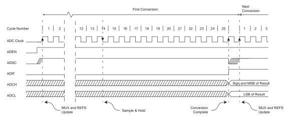
The actual sample-and-hold takes place 1.5 ADC clock cycles after the start of a normal conversion and 13.5 ADC clock cycles after the start of an first conversion. See Figure 15-5.
