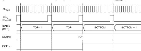
Figure 11-10. Timer/Counter Timing Diagram, CTC mode, with Prescaler (f<sub>clk I/O</sub>/8)
