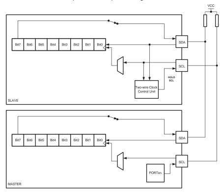
Figure 13-4. Two-wire Mode Operation, Simplified Diagram
