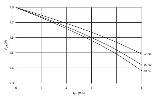
**Figure 20-30.**  $V_{OH}$ : Output Voltage vs. Source Current (I/O Pin,  $V_{CC} = 3V$ )
