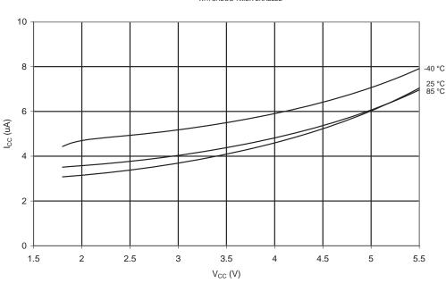
POWER-DOWN SUPPLY CURRENT vs. SUPPLY VOLTAGE WATCHOOG TIMER ENABLED
