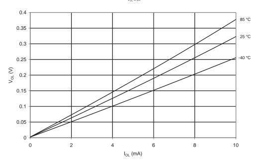
Figure 20-130.  $V_{OL}$ : Output Voltage vs. Sink Current (I/O Pin,  $V_{CC}$  = 5V)
