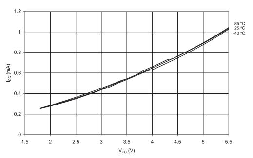
Figure 20-56. Active Supply Current vs. V<sub>CC</sub> (Internal Calibrated Oscillator, 128 kHz)
