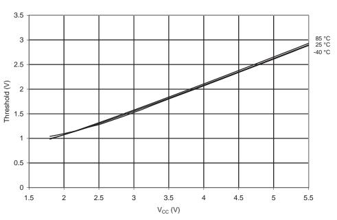
Figure 20-88. V<sub>IL</sub>: Input Threshold Voltage vs. V<sub>CC</sub> (I/O Pin, Read as '0')
