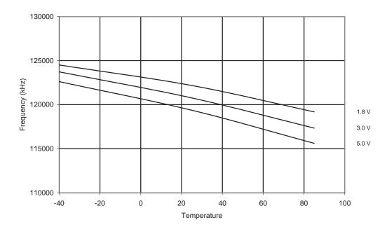
Figure 20-49. Frequency of Calibrated 8.0 MHz Oscillator vs. V<sub>CC</sub>
