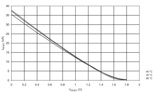
**Figure 20-75.** Pull-Up Resistor Current vs. Input Voltage (Reset Pin,  $V_{CC} = 3V$ )
