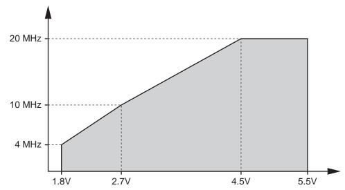
Figure 19-1. Maximum Operating Frequency vs. Supply Voltage
