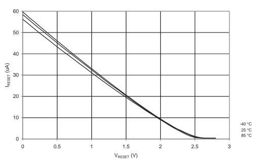
**Figure 20-76.** Pull-Up Resistor Current vs. Input Voltage (Reset Pin,  $V_{CC} = 5V$ )
