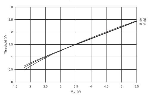
**Figure 20-140.**  $V_{IH}$ - $V_{IL}$ : Input Hysteresis vs.  $V_{CC}$  (I/O Pin)
