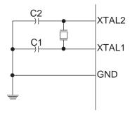
C1 and C2 should always be equal for both crystals and resonators. The optimal value of the capacitors depends on the crystal or resonator in use, the amount of stray capacitance, and the electromagnetic noise of the environment. Some initial guidelines for choosing capacitors for use with crystals are given in Table 6-11. For ceramic resonators, the capacitor values given by the manufacturer should be used.
