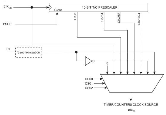
Note: 1. The synchronization logic on the input pins (T0) is shown in Figure 11-3.
