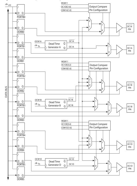
Figure 12-10. Compare Match Output Unit, Schematic
