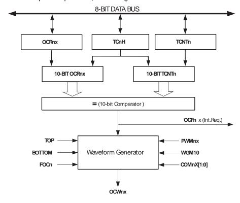
The OCR1x Registers are double buffered when using any of the Pulse Width Modulation (PWM) modes. For the normal mode of operation, the double buffering is disabled. The double buffering synchronizes the update of the OCR1x Compare Registers to either top or bottom of the counting sequence. The synchronization prevents the occurrence of odd-length, non-sym-
