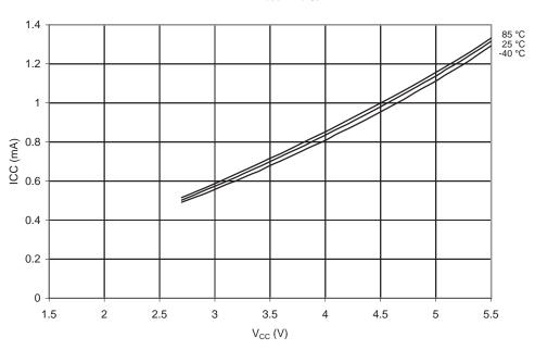
$\textbf{Figure 20-60.} \quad \text{Idle Supply Current vs. V}_{\text{CC}} \text{ (Internal Calibrated Oscillator, 1 MHz)}$
