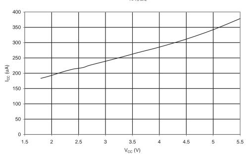
Figure 20-119. Timer/Counter1 Current vs.  $V_{CC}$
