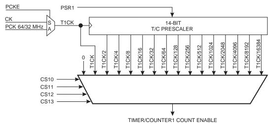
In the asynchronous clocking mode the clock selections are from PCK to PCK/16384 and stop, and in the synchronous clocking mode the clock selections are from CK to CK/16384 and stop. The clock options are illustrated in Figure 12-3 and desribed in "TCCR1B – Timer/Counter1 Control Register B" on page 114.
