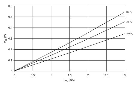
Figure 20-135.  $V_{OL}$ : Output Voltage vs. Sink Current (Reset Pin as I/O, T = 25°C)
