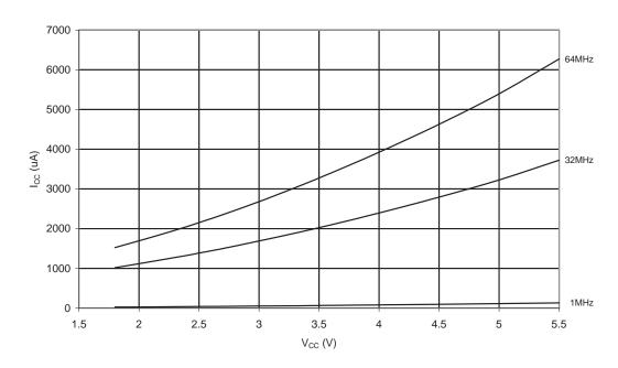
Figure 20-69. Brownout Detector Current vs. V<sub>CC</sub>
