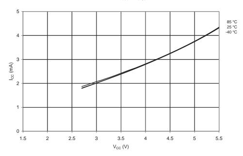
$\textbf{Figure 20-4.} \qquad \text{Active Supply Current vs. V}_{\text{CC}} \text{ (Internal Calibrated Oscillator, 1 MHz)}$
