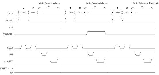
**Figure 18-7.** Programming the FUSES Waveforms
