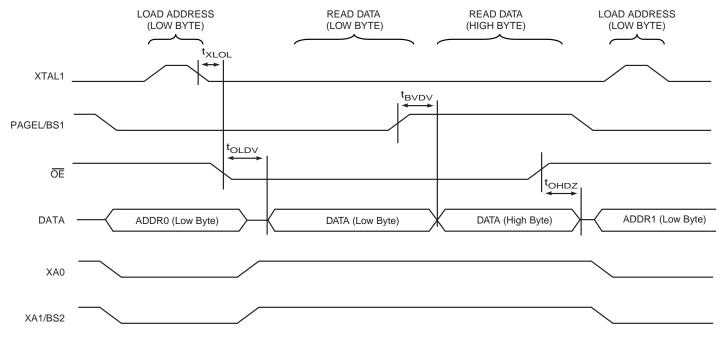
Note: The timing requirements shown in Figure 19-5 (i.e., t<sub>DVXH</sub>, t<sub>XHXL</sub>, and t<sub>XLDX</sub>) also apply to reading operation.
