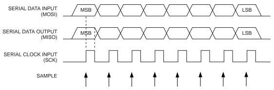
Figure 19-4. Serial Programming Timing
