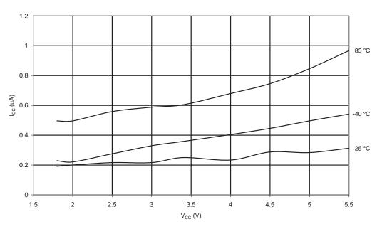
Figure 20-63. Power-down Supply Current vs. V<sub>CC</sub> (Watchdog Timer Enabled)
