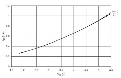
Figure 20-107. Active Supply Current vs. V<sub>CC</sub> (Internal Calibrated Oscillator, 128 kHz)
