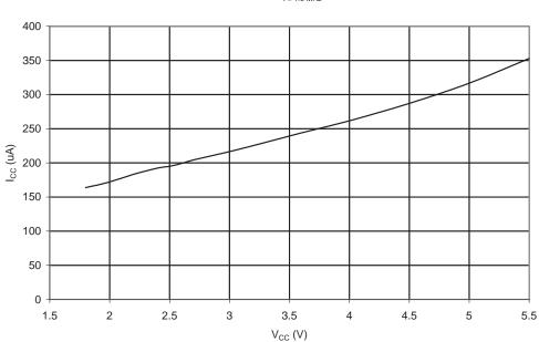
Figure 20-68. Timer/Counter1 Current vs. V<sub>CC</sub>
