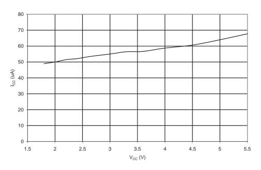
Figure 20-118. ADC Current vs.  $V_{CC}$  (AREF =  $AV_{CC}$ )
