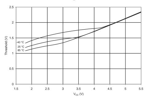
**Figure 20-40.**  $V_{IL}$ : Input Threshold Voltage vs.  $V_{CC}$  (Reset Pin, Read as '0') RESET INPUT THRESHOLD VOLTAGE vs. VCC
