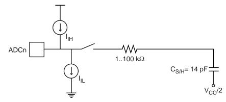
The capacitor in Figure 15-8 depicts the total capacitance, including the sample/hold capacitor and any stray or parasitic capacitance inside the device. The value given is worst case.
