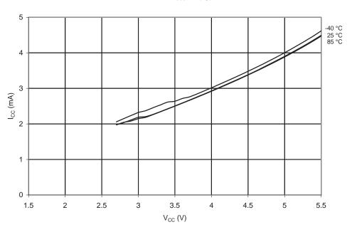
$\textbf{Figure 20-106.} \ \, \textbf{Active Supply Current vs. V}_{\text{CC}} \ \, \textbf{(Internal Calibrated Oscillator, 1 MHz)}$
