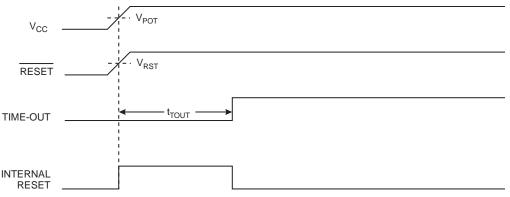
Figure 8-3. MCU Start-up, RESET Extended Externally
