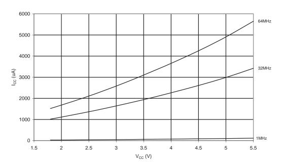
Figure 20-120. Brownout Detector Current vs.  $V_{CC}$
