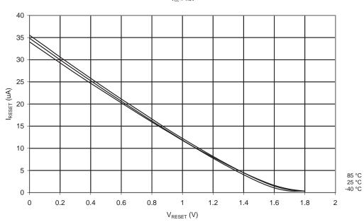
**Figure 20-24.** Pull-Up Resistor Current vs. Input Voltage (Reset Pin,  $V_{CC} = 3V$ )
