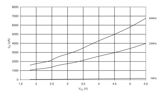
Figure 20-18. Brownout Detector Current vs.  $V_{CC}$
