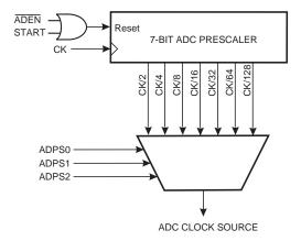
The ADC module contains a prescaler, which generates an acceptable ADC clock frequency from any CPU frequency above 100 kHz. The prescaling is set by the ADPS bits in ADCSRA. The prescaler starts counting from the moment the ADC is switched on by setting the ADEN bit in ADCSRA. The prescaler keeps running for as long as the ADEN bit is set, and is continuously reset when ADEN is low. See Figure 15-3.
