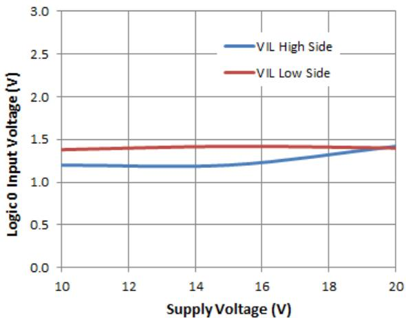
**Figure 22.** Logic 0 Input Voltage vs. Supply Voltage
