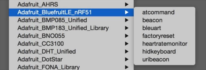
This will open up a new instance of the example in the IDE, as shown below. You can edit the URL that the beacon will point to, from the default <http://www.adafruit.com> or just upload as is to test
