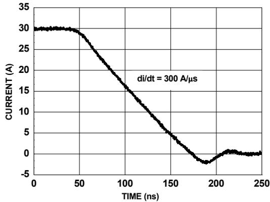
Figure 14. FDMS7560S SyncFET body diode reverse recovery characteristic
