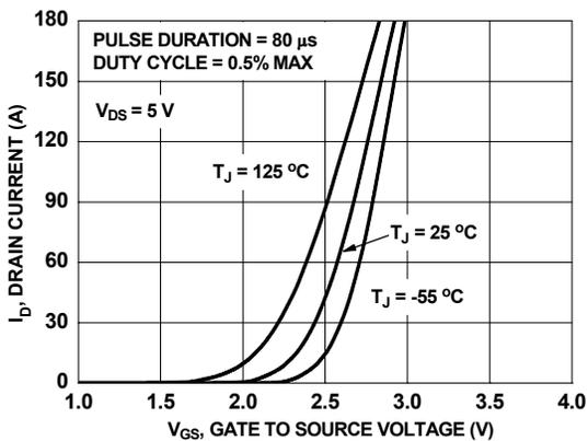
**Figure 5. Transfer Characteristics**
