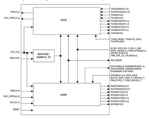
Supports the physical link layer of the OBSAI RP3 specification
