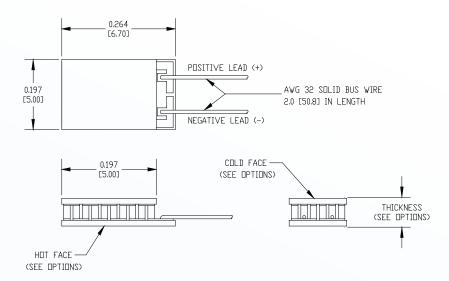
Ceramic Material 96% Alumina Ceramics Solder Construction: 138°C, Bismuth Tin
