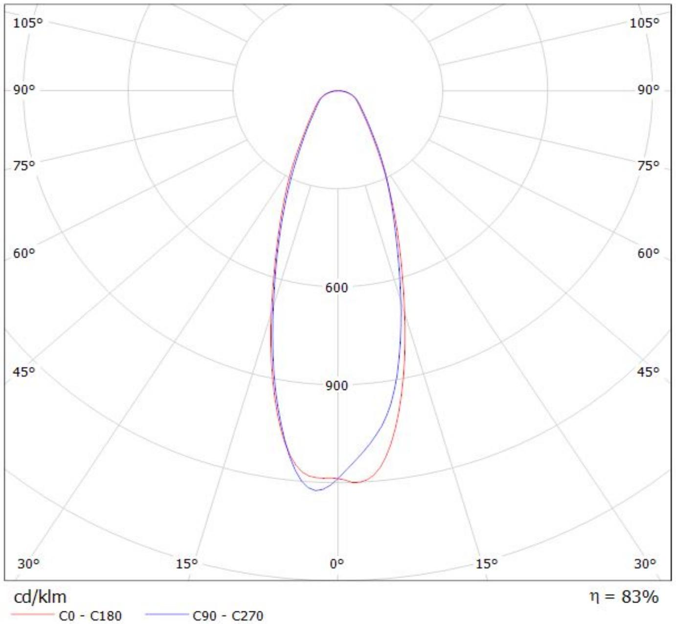
Luminaire: Ledil FN15679\_RONDA-S\_(MJT\_30W\_Les14,5)\_TE
