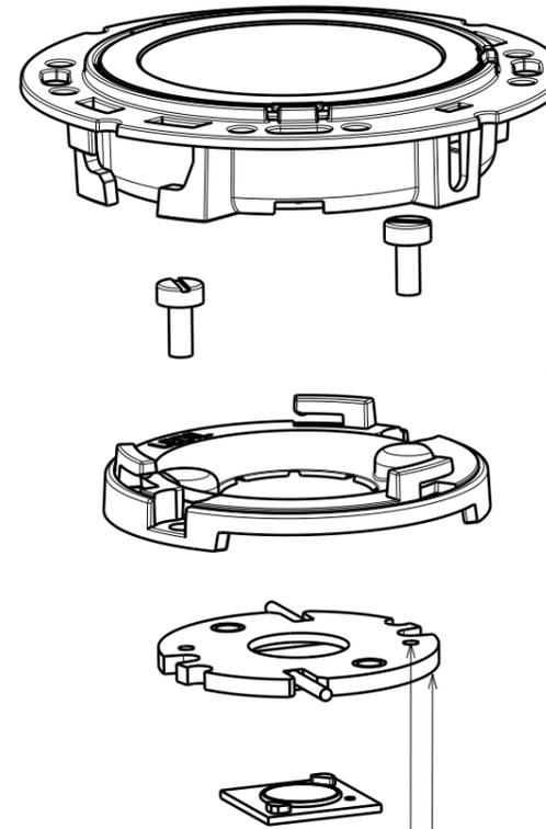
1. Ensure correct relation of clamp and connector before screwing. Recommended torque 0.6Nm.
