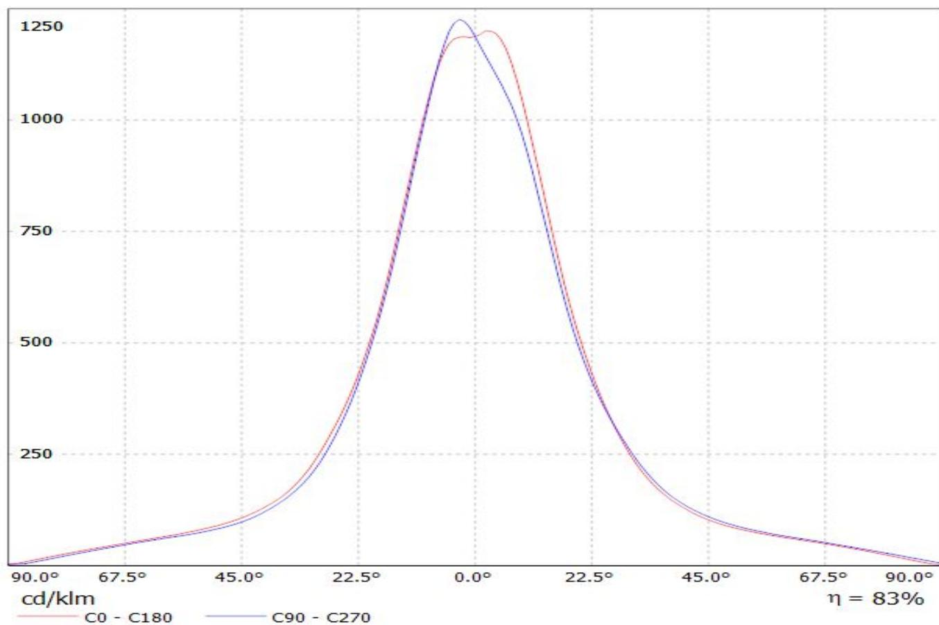
Luminaire: Ledil FN15679\_RONDA-S\_(MJT\_30W\_Les14,5)\_TE
