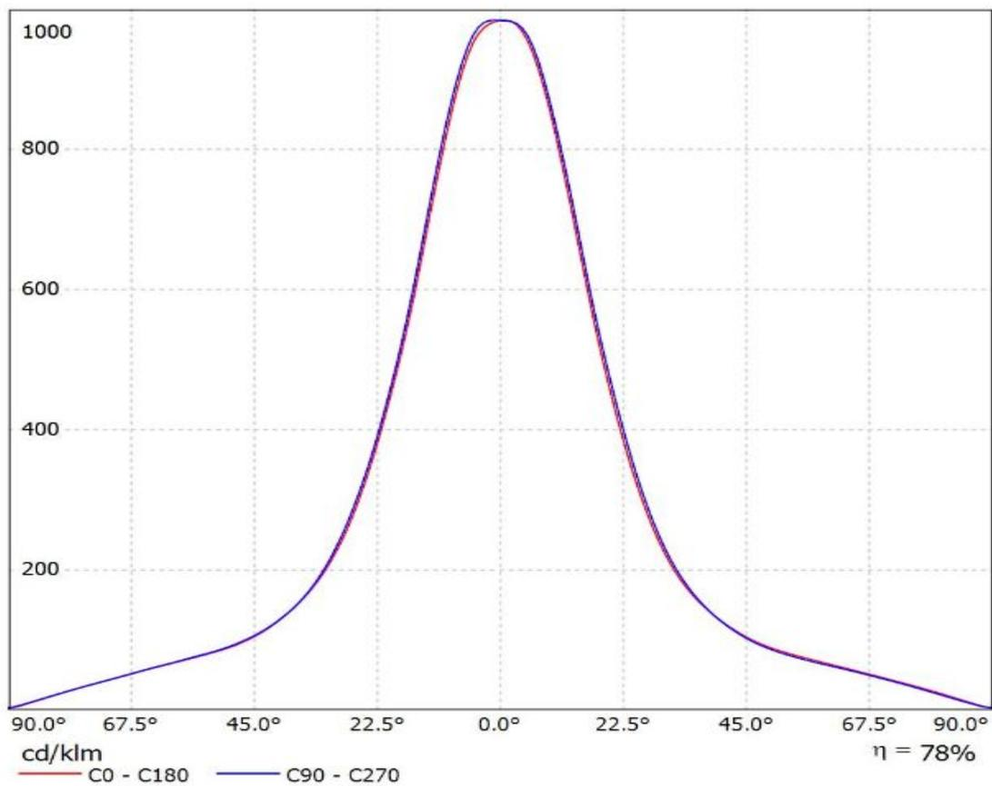
Luminaire: Ledil Oy PRELIMINARY\_FN15679\_RONDA-S\_(SLE\_G6\_LES15)\_(2213254-2+\_2213194-1)
