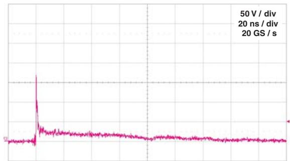
**Figure 7. ESD response to IEC 61000-4-2 (-8 kV contact discharge)**
