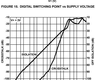
FREQUENCY (Hz) FIGURE 17. CROSSTALK AND OFF ISOLATION
