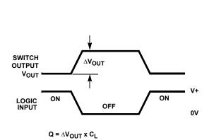
FIGURE 2A. MEASUREMENT POINTS
