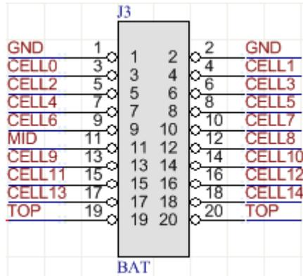
Figure 3: Battery Connector
