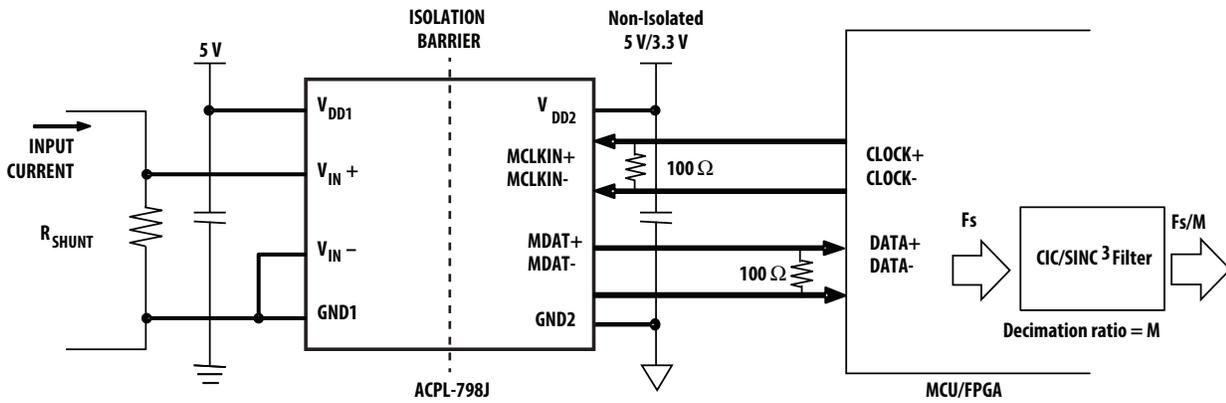
Note: In applications, a 0.1  $\mu\text{F}$  bypass capacitor must be connected between pins  $V_{DD1}$  and  $GND1$ , and between pins  $V_{DD2}$  and  $GND2$  of the ACPL-798J.
