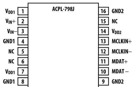
Figure 2. Pin configuration.
