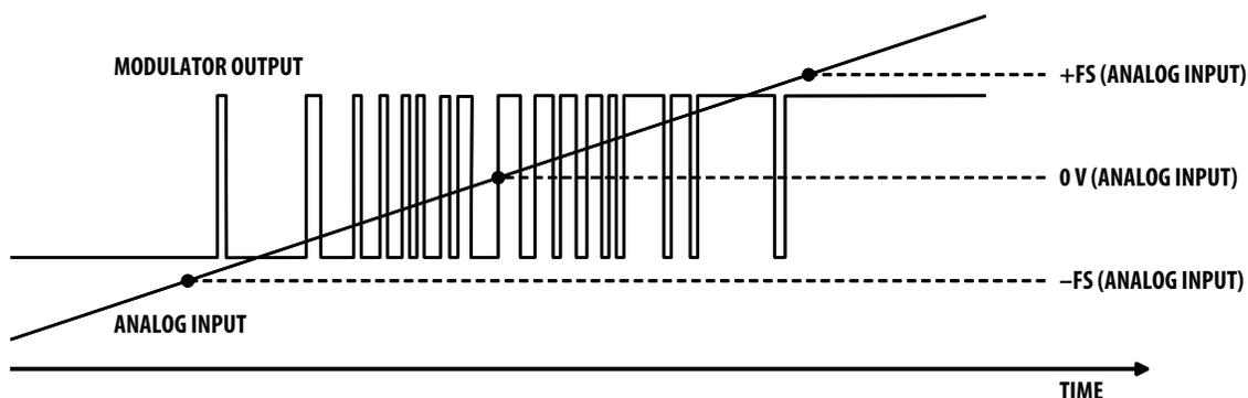
Figure 24. Modulator output vs. analog input.
