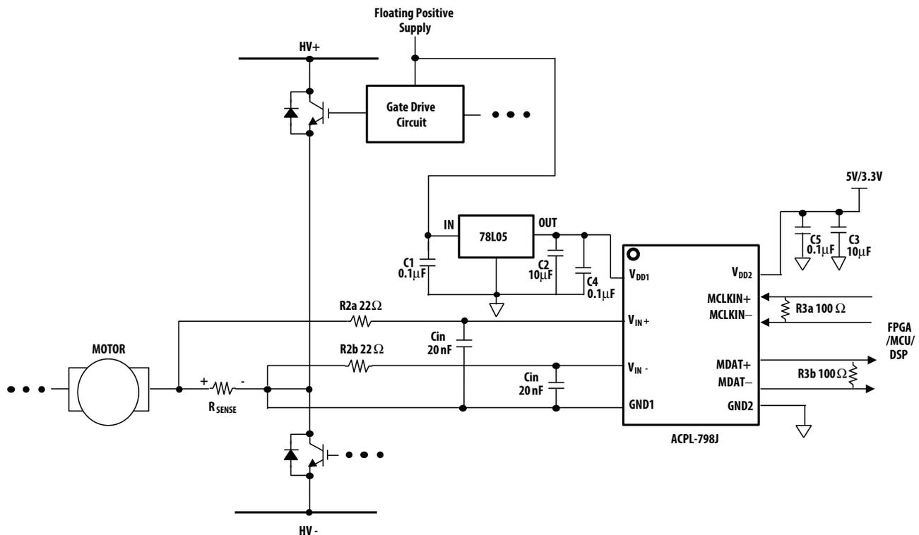
**Figure 28. Schematic for three conductor shunt connection.**
