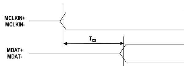
**Figure 5. Data delay upon clock input startup**
