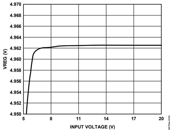
Figure 9. V<sub>REG</sub> vs. Input Voltage, 10 mA Load
