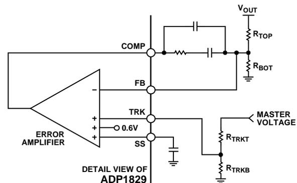
Figure 30. Voltage Tracking
