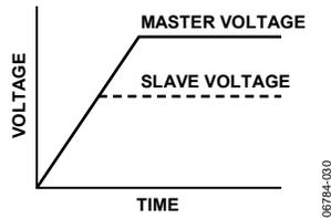
Figure 31. Coincident Tracking
