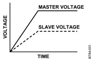
Figure 32. Ratiometric Tracking
