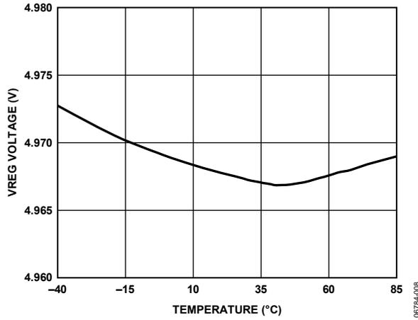
Figure 8. V<sub>REG</sub> Voltage vs. Temperature
