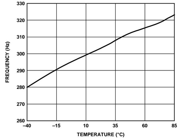
Figure 14. Switching Frequency vs. Temperature,  $V_{IN} = 12\text{ V}$
