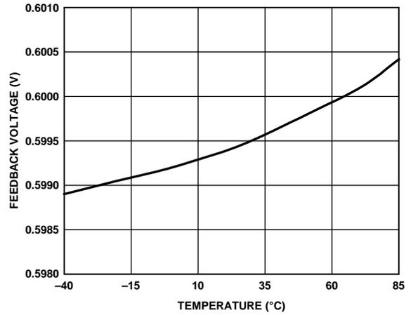
Figure 13. Feedback Voltage vs. Temperature,  $V_{IN} = 12\text{ V}$
