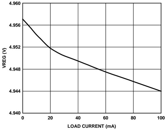
Figure 10. VREG vs. Load Current,  $V_{IN} = 12\text{ V}$
