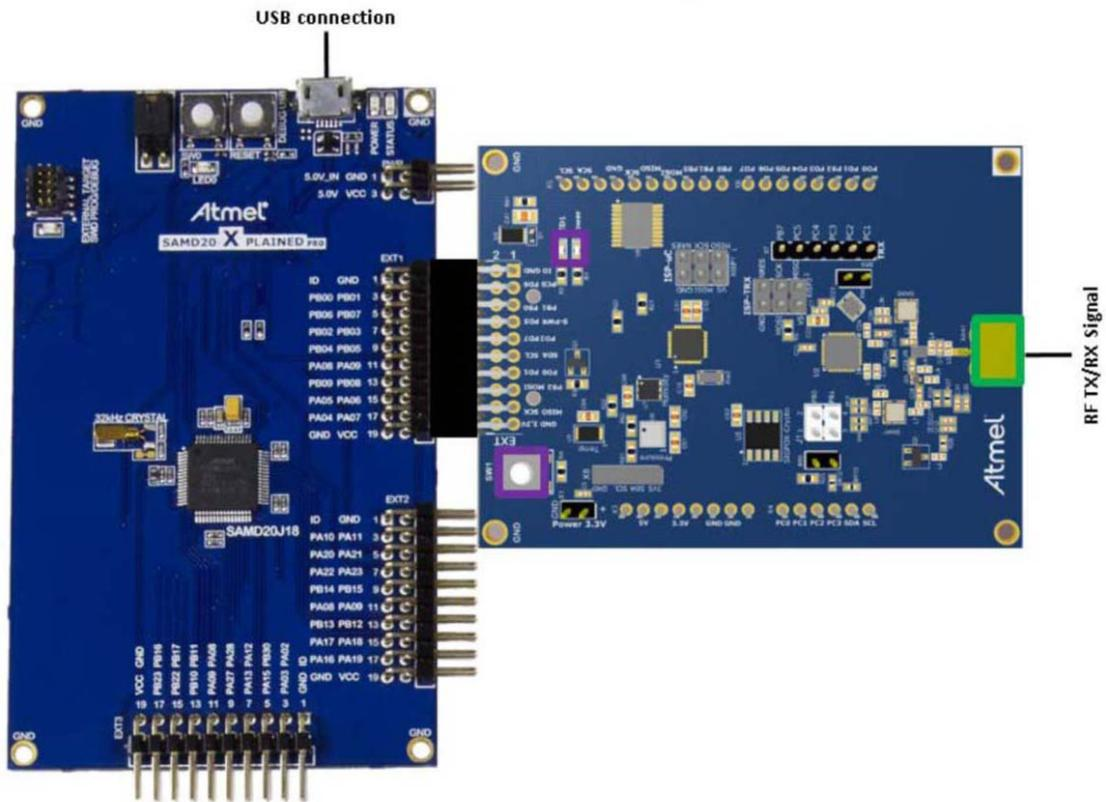
The 868MHz monopole antenna is connected to the SMA connector of the PCB and the board is powered from the attached evaluation kit using 3V/5V for the ATA8520-EK2-E Xplained Mini and 3V for the ATA8520-EK3-E Xplained Pro.
