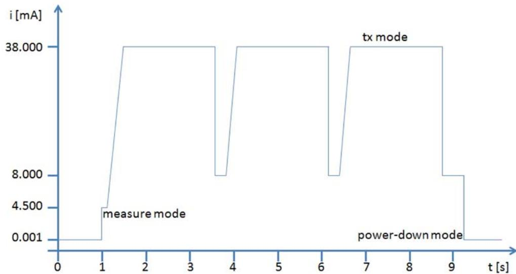
[Table 5-1](#) summarizes battery service life for a typical Lithium battery which can be used with the ATAB0101A. When selecting the battery, it is important to know the peak current consumption which has to be supplied by the battery cells. It is assumed that the battery voltage drops from the initial value of 3V down to 2V at the end of its service life. The self-discharge is defined by the manufacturer as typically 1% per year at an ambient temperature of 20°C.
