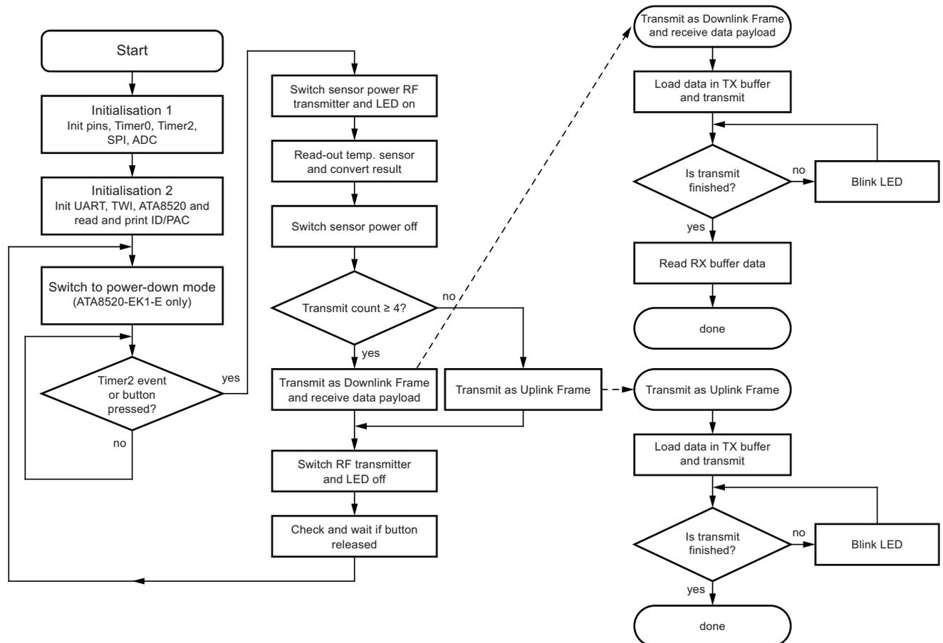
During the step Initialisation1 the application will perform a check for the device version to be V1.3. This device version supports the temperature drift calibration and includes fixes for the test function. Previous device version will not support this modes
