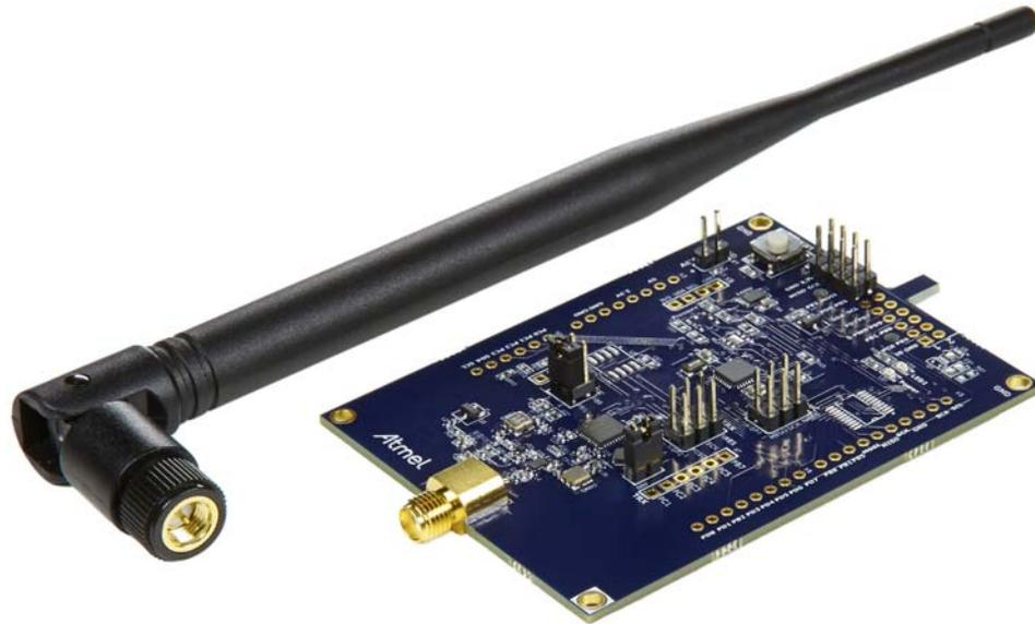
The 868MHz monopole antenna is connected to the SMA connector of the PCB and the external power supply or battery has to be connected to connector X1.
