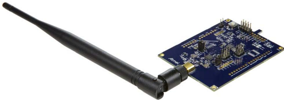
Figure 2-2. ATA8520-EK2-E Xplained Mini Extension Board Mounted on Xplained Mini
