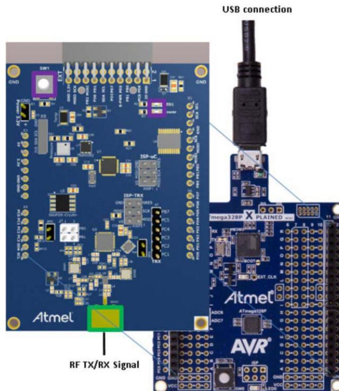
Figure 2-3. ATA8520-EK3-E Xplained Pro Extension Board
