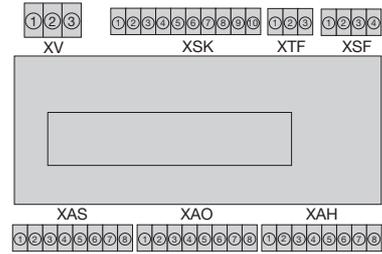
Wire size: 0.14 mm<sup>2</sup> to 1.5 mm<sup>2</sup> single or stranded conductor
