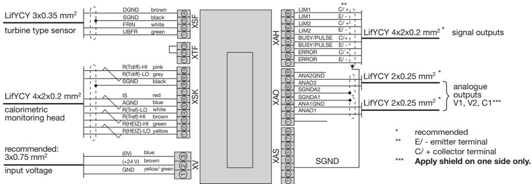
**FM1 - Recommended connection of pulse output**
