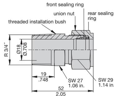
Suitable up to 25 bar/2.5 M Pascal if used with stainless steel CSF-01 monitoring head.
