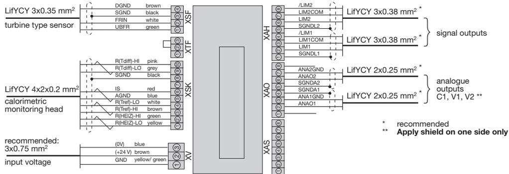
**FM1 with transistor outputs**
