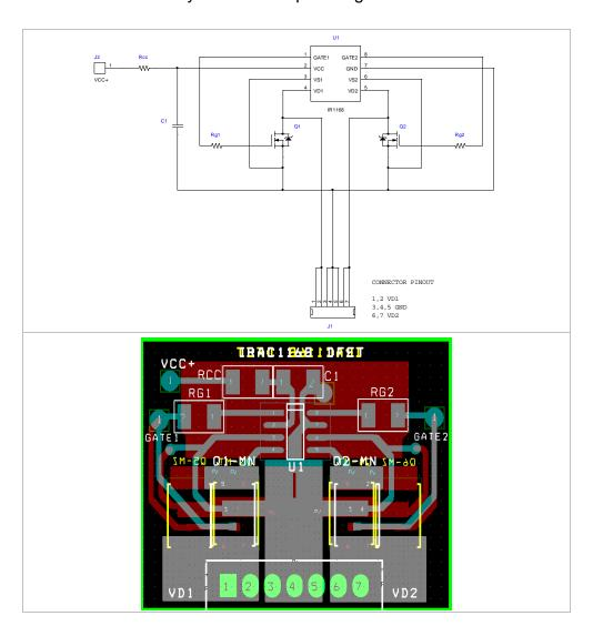
The daughter card shown above is designed to allow easy retrofit in existing systems with minimal system changes. For the DFET daughter card shown above, there are multiple footprints for the synchronous rectifier MOSFETs to accommodate three different medium can DFET packages (MN, MT and MZ).
