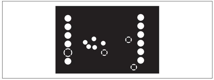
Figure 4. MAX5487PMB1 Peripheral Module PCB Layout—Inner Layer 1 (Ground)
