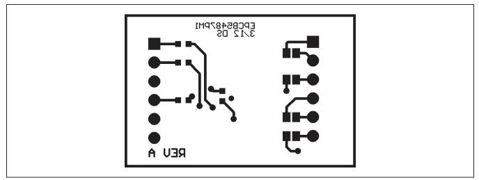
Figure 6. MAX5487PMB1 Peripheral Module PCB Layout—Solder Side
