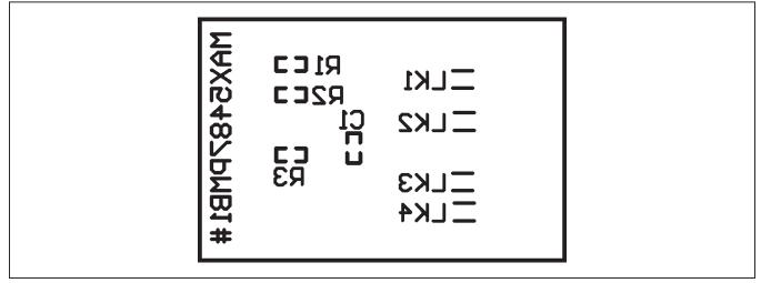
Figure 7. MAX5487PMB1 Peripheral Module Component Placement Guide—Solder Side
