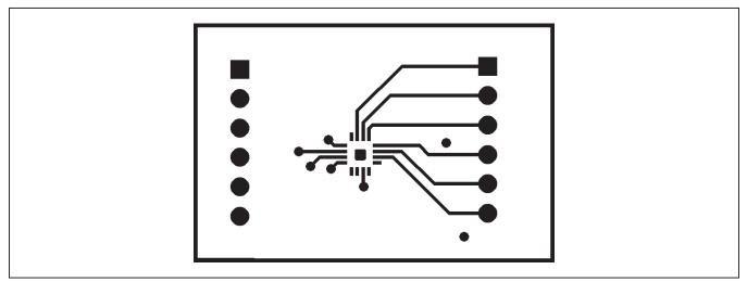
Figure 3. MAX5487PMB1 Peripheral Module PCB Layout—Component Side
