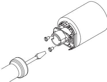
1. Fasten the Base on the motor (Tool C may need to be rotated to allow for some mounting configurations).
