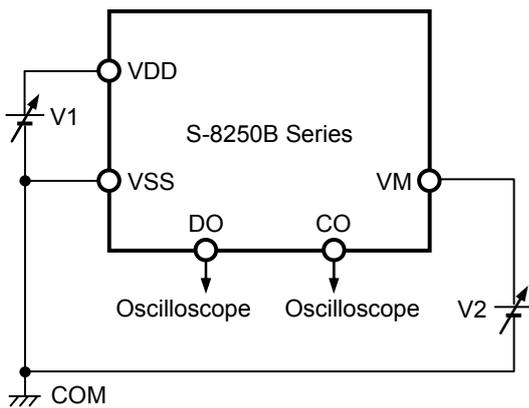
**Figure 8 Test Circuit 5**
