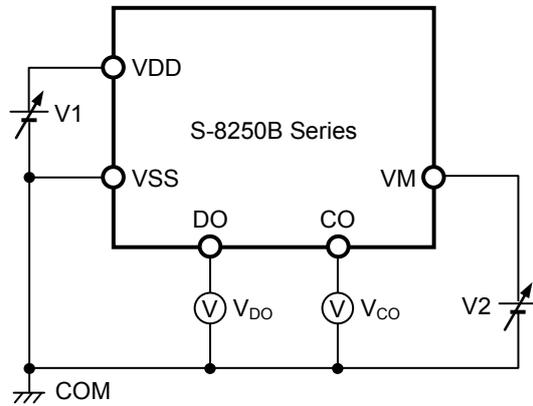
**Figure 5 Test Circuit 2**
