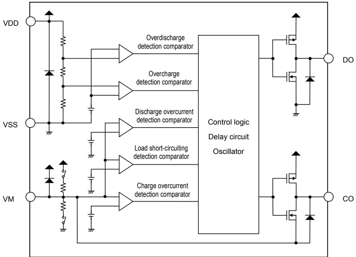
**Remark** All the diodes shown in the figure are parasitic diodes.
