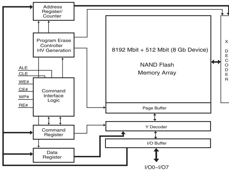
**Figure 4.2** Block Diagram — 1 CE (4 Gb x 8)
