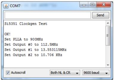
Now you can use your oscilloscope to probe the #0, #1 and #2 outputs Depending on your oscillioscope make and model, it may not be possible for you to verify the 112.5MHz output frequency!
