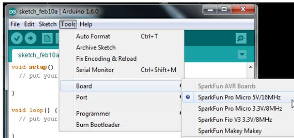
Notice there are two options for Pro Micro - 8MHz and 16MHz. It’s very important that you **select the Pro Micro option that matches your board’s voltage and speed**. Don’t know which board you have? Check the bottom of the board, where you should find either a ‘5V’ or ‘3.3V’ box checked.
