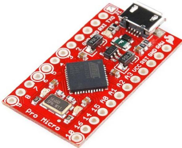
The SparkFun Pro Micro is a really cool, little development board. It's an Arduino-compatible microcontroller, micro-sized, and it accomplishes with one single chip what old Arduino Unos, Duemilanoves, and Diecimeillas could never dream of: true USB functionality.
