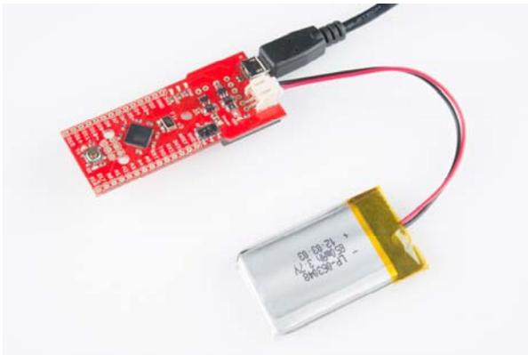
The 'CHG' LED will indicate the status of the battery charge. If it's on, the battery is still charging. Once the 'CHG' LED goes off, the battery is fully charged.
