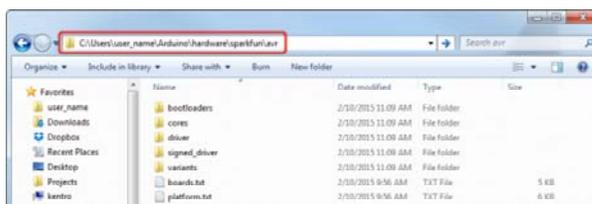
The structure of this directory is critical – it should look something like “Arduino/hardware/[manufacturer]/[architecture]”, in this case [manufacturer] is “sparkfun”, and [architecture] is “avr.”
