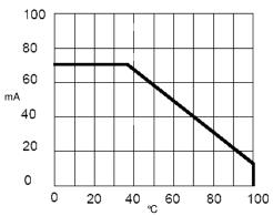
Maximum Forward DC Current vs Ambient Temperature
