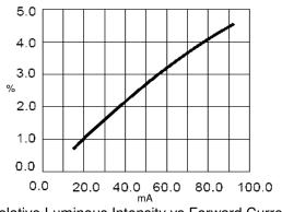
Relative Luminous Intensity vs Forward Current
