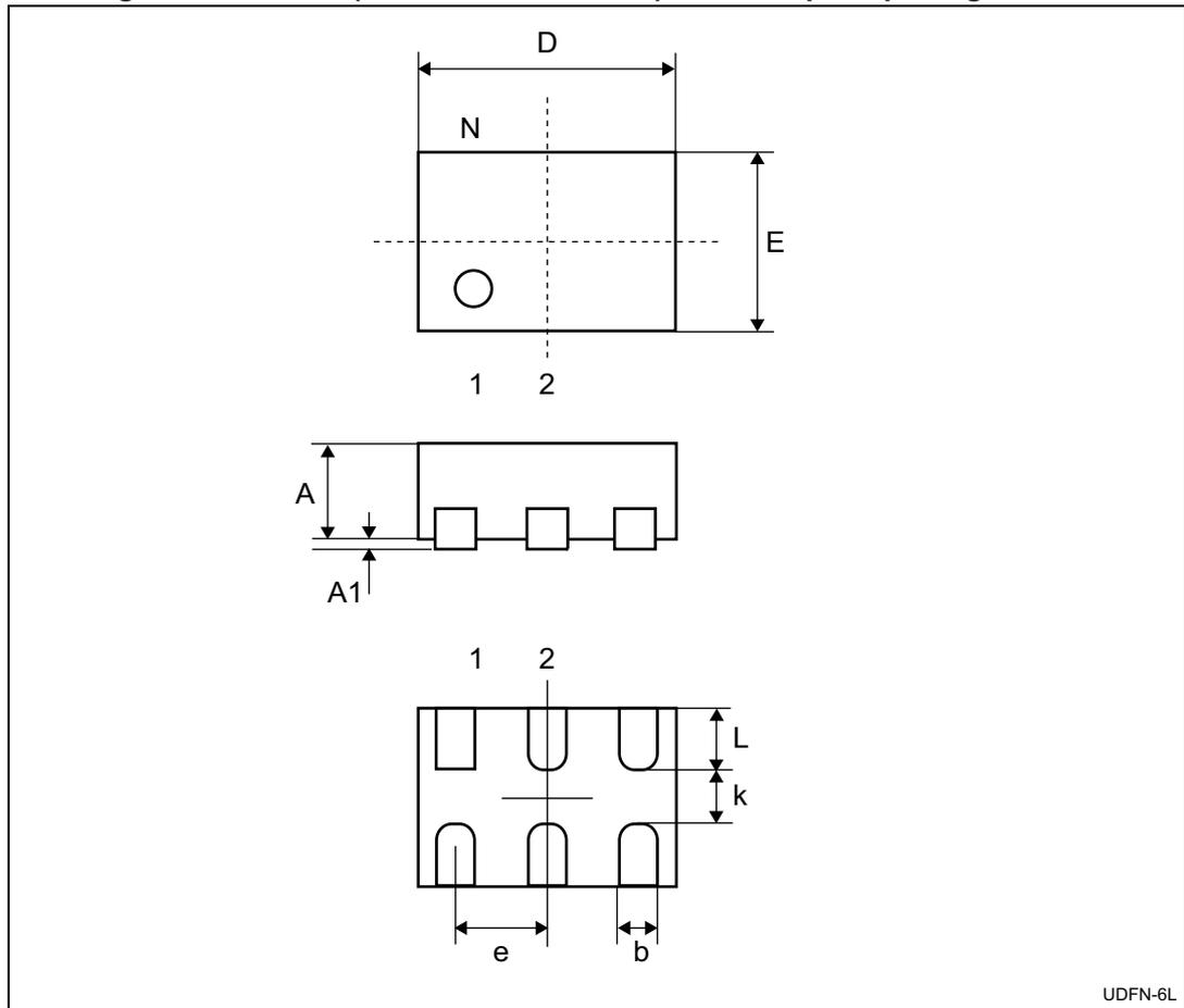
**Table 5. UDFN6, (1.00 x 1.45 x 0.50 mm), 0.50 mm pitch package mechanical data**
