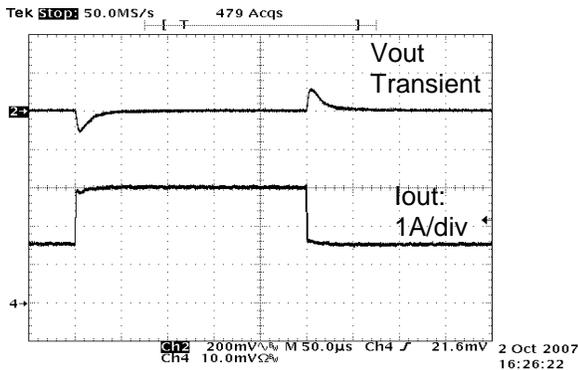
Figure 5. Load Step Response 1.5->3A
