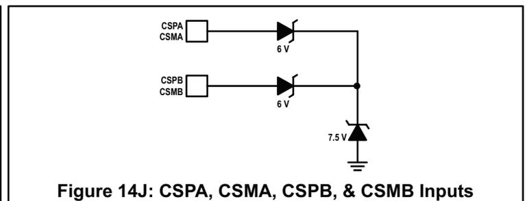
Figure 14J: CSPA, CSMA, CSPB, & CSMB Inputs
