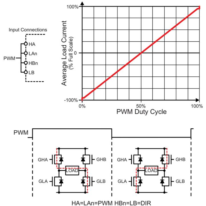
Figure 10: Single PWM Input, Fast Decay, SR
