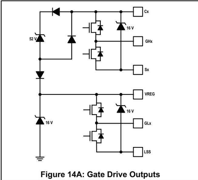
Figure 14A: Gate Drive Outputs
