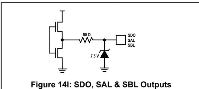
Figure 14I: SDO, SAL & SBL Outputs
