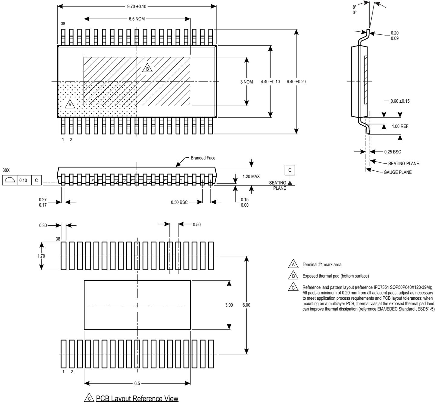
Figure 15: Package LV, 38-Pin eTSSOP with Exposed Pad
