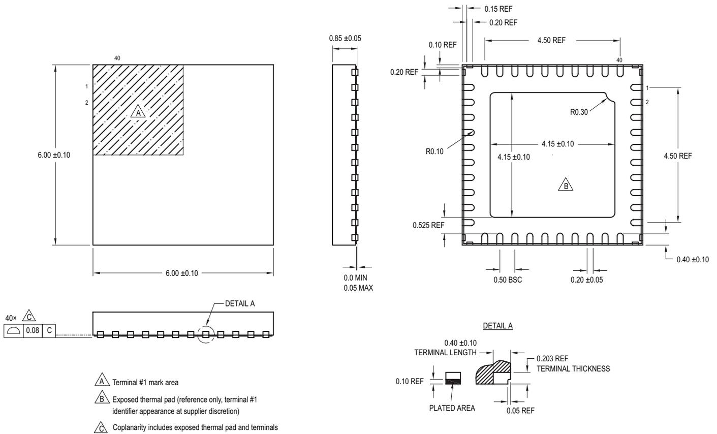
Figure 16: Package EV, Wettable Flank 40-Terminal eQFN with Exposed Pad
