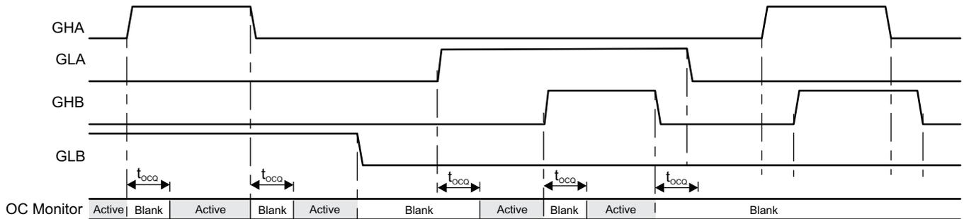
Figure 4: Overcurrent Fault Monitor – Blank Mode Timing (OCQ=1)
