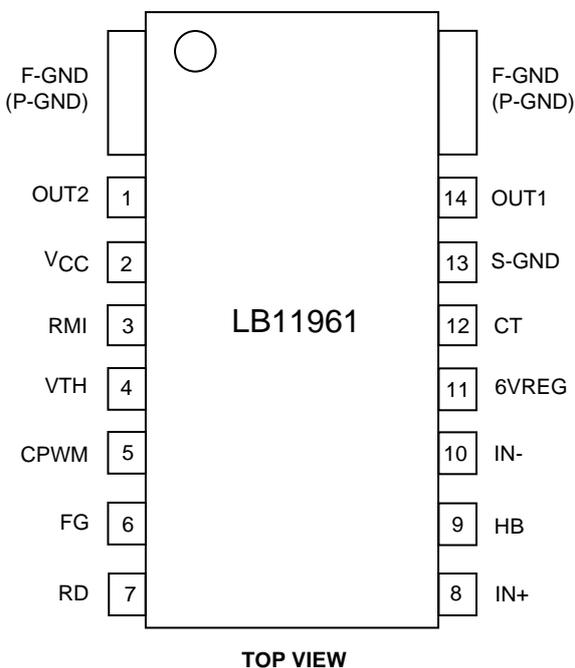
F-GND (P-GND) : The motor system ground and the heat sink. Since the heat generated by the chip is dissipated through F-GND, the thermal resistance is lowered by increasing the area of the copper foil and solder surface in the printed circuit pattern.
