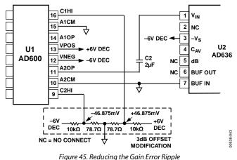
The error curve shown in Figure 46 demonstrates that, over the central portion of the range, the output voltage can be maintained close to the ideal value. The penalty for this modification is higher errors at the extremities of the range. The next two applications show how three amplifier sections can be cascaded to extend the nominal conversion range to 120 dB, with the inclusion of simple LP filters of the type shown in Figure 37. Very low errors can then be maintained over a 100 dB range.
