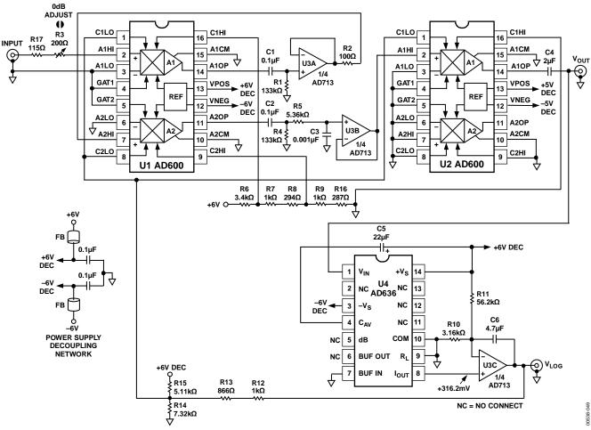
Figure 51. 120 dB Dynamic Range RMS Responding Circuit Optimized for SNR
