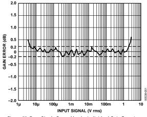
Figure 53. Error Ripple Caused by the Individual Gain Functions
