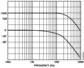
Figure 5. AD602 Frequency and Phase Response vs. Gain
