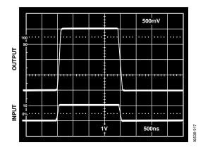
Figure 17. Transient Response Minimum Gain
