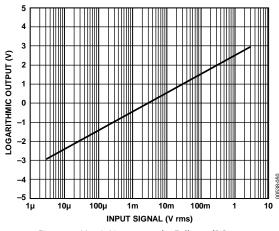
Figure 52. V<sub>LOG</sub> Is Linear over the Full 120 dB Range
