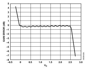
Figure 28. Gain Error for Cascaded Stages—Sequential Control
