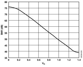
Figure 32. SNR vs. Control Voltage—Low Ripple Mode
