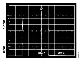
Figure 14. Transient Response, Medium and High Gain
