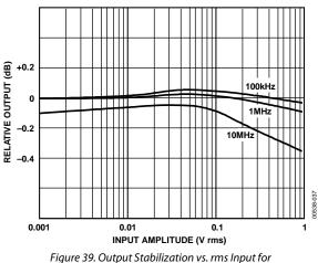
Figure 39. Output Stabilization vs. rms Input for Sine Wave Inputs at 100 kHz, 1 MHz, and 10 MHz
