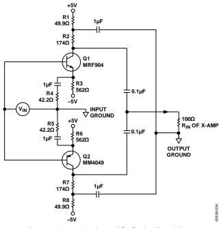
Figure 36. A Low Noise Preamplifier for the AD600/AD602
