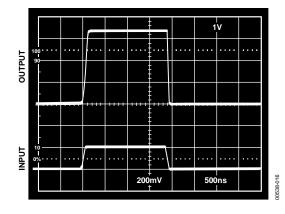
Figure 16. Output Stage Overload Recovery Time
