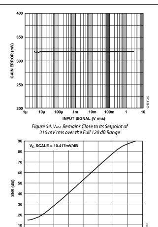
V<sub>C</sub> (mV) Figure 55. SNR vs. Control Voltage for Parallel Gain Control (See Figure 47)
