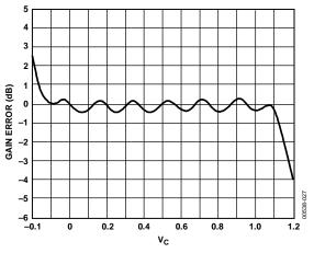
Figure 29. Gain Error for Cascaded Stages—Parallel Control
