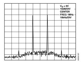
Figure 7. Third-Order Intermodulation Distortion,  $V_{OUT} = 2 V p$ -p,  $R_L = 500 \Omega$
