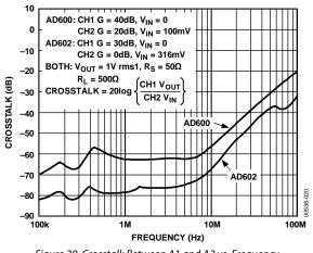
Figure 20. Crosstalk Between A1 and A2 vs. Frequency
