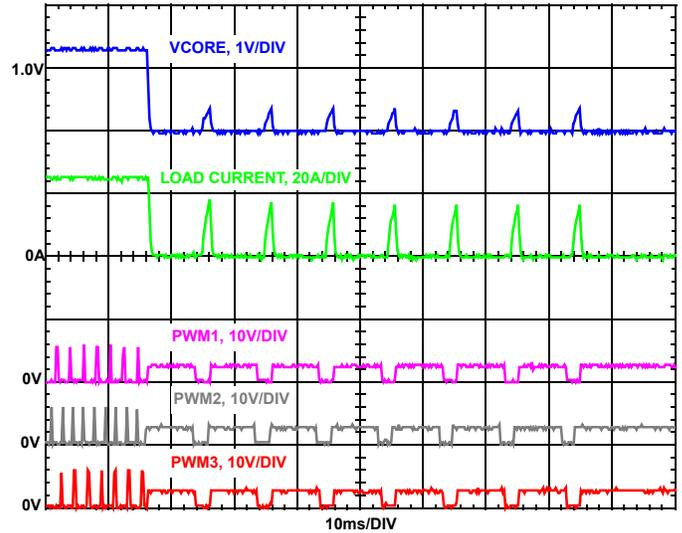
FIGURE 5. OVER-CURRENT PROTECTION
