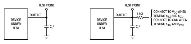
\*Includes all probe and jig capacitance
