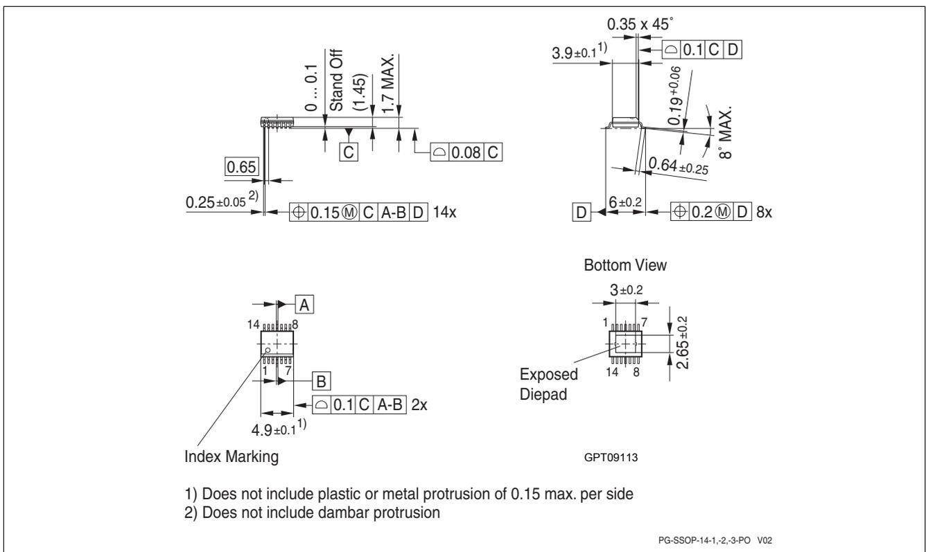
Figure 6 PG-SSOP-14
