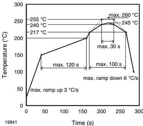
Fig. 7 - Lead (Pb)-free Reflow Solder Profile acc. J-STD-020
