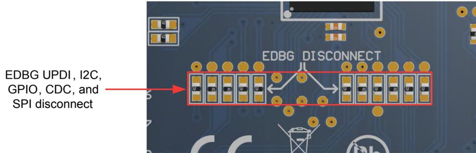
Figure 4-7. ATtiny817 Xplained Pro Current Measurement Headers
