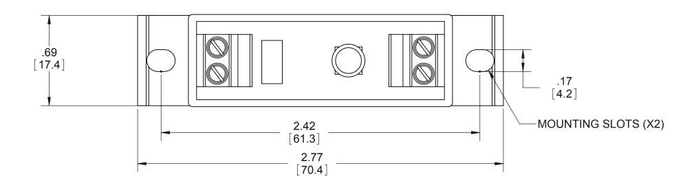
Tolerances: ± 0.02 in / 0.5 mm. All dimensions are in: inches [millimeters]
