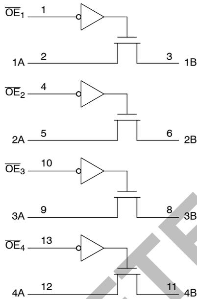
Figure 3. Logic Diagram
