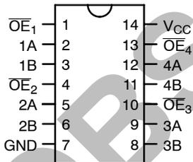
Figure 1. Pin Assignment for SOIC and TSSOP
