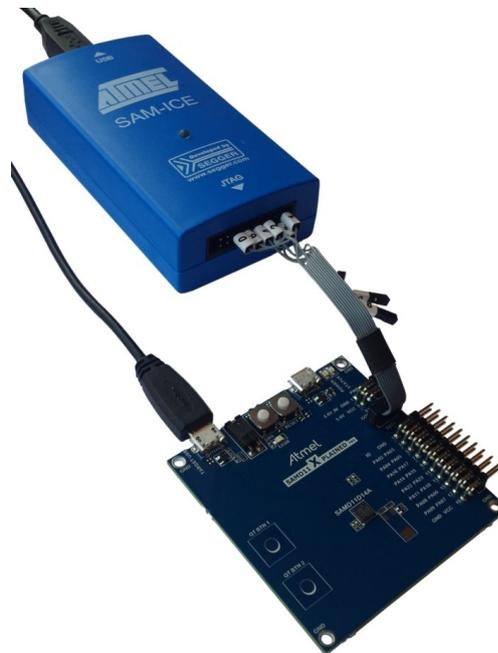
Figure 5-7. SAM-ICE using an Atmel-ICE Adapter
