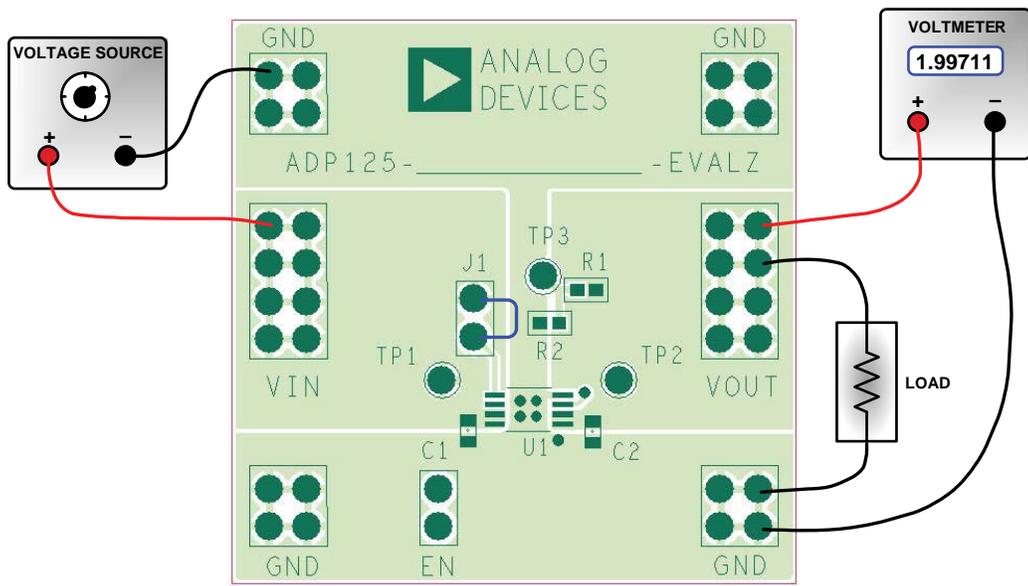
Figure 8. ADP125 Output Voltage Measurement Setup, MSOP
