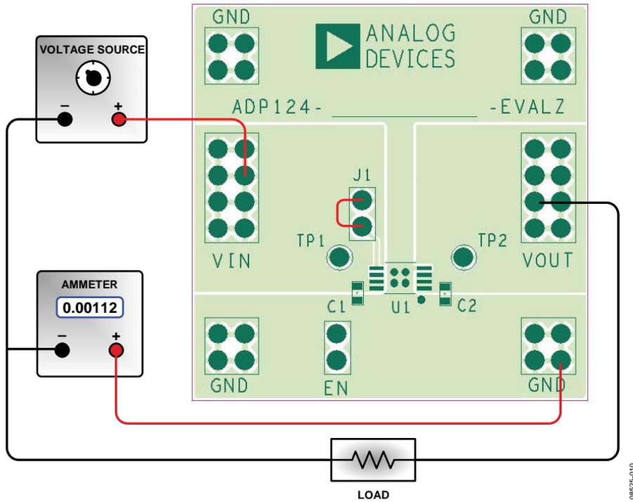
Figure 13. ADP124 Ground Current Measurement Setup, MSOP
