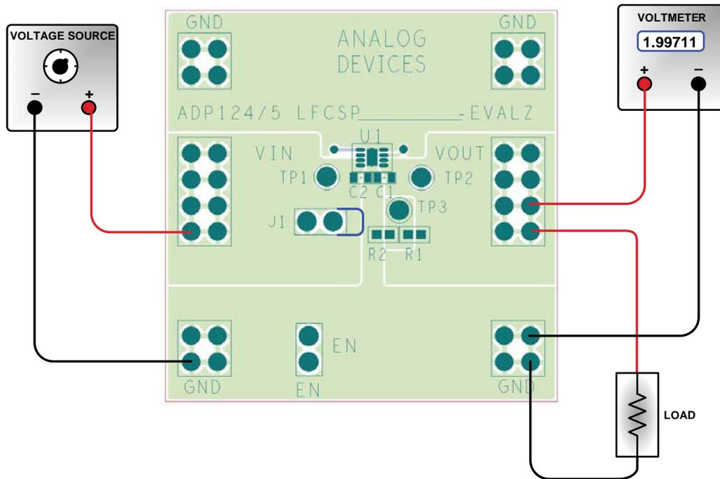
Figure 9. ADP124/ADP125 Output Voltage Measurement Setup, LFCSP
