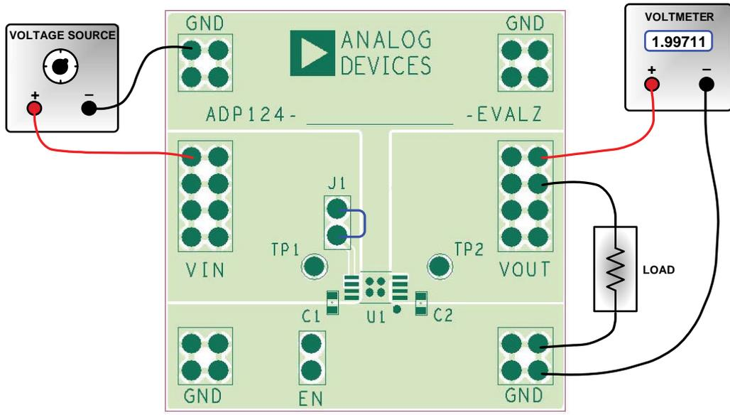
Figure 7. ADP124 Output Voltage Measurement Setup, MSOP
