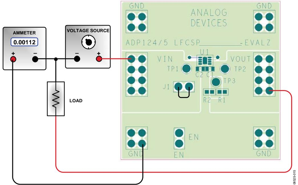
Figure 15. ADP124/ADP125 Ground Current Measurement Setup, LFCSP
