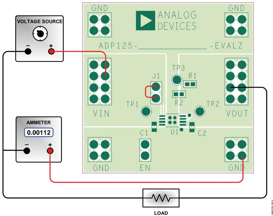
Figure 14. ADP125 Ground Current Measurement Setup, MSOP
