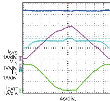
**Input Voltage Clamp, Charge Mode**
