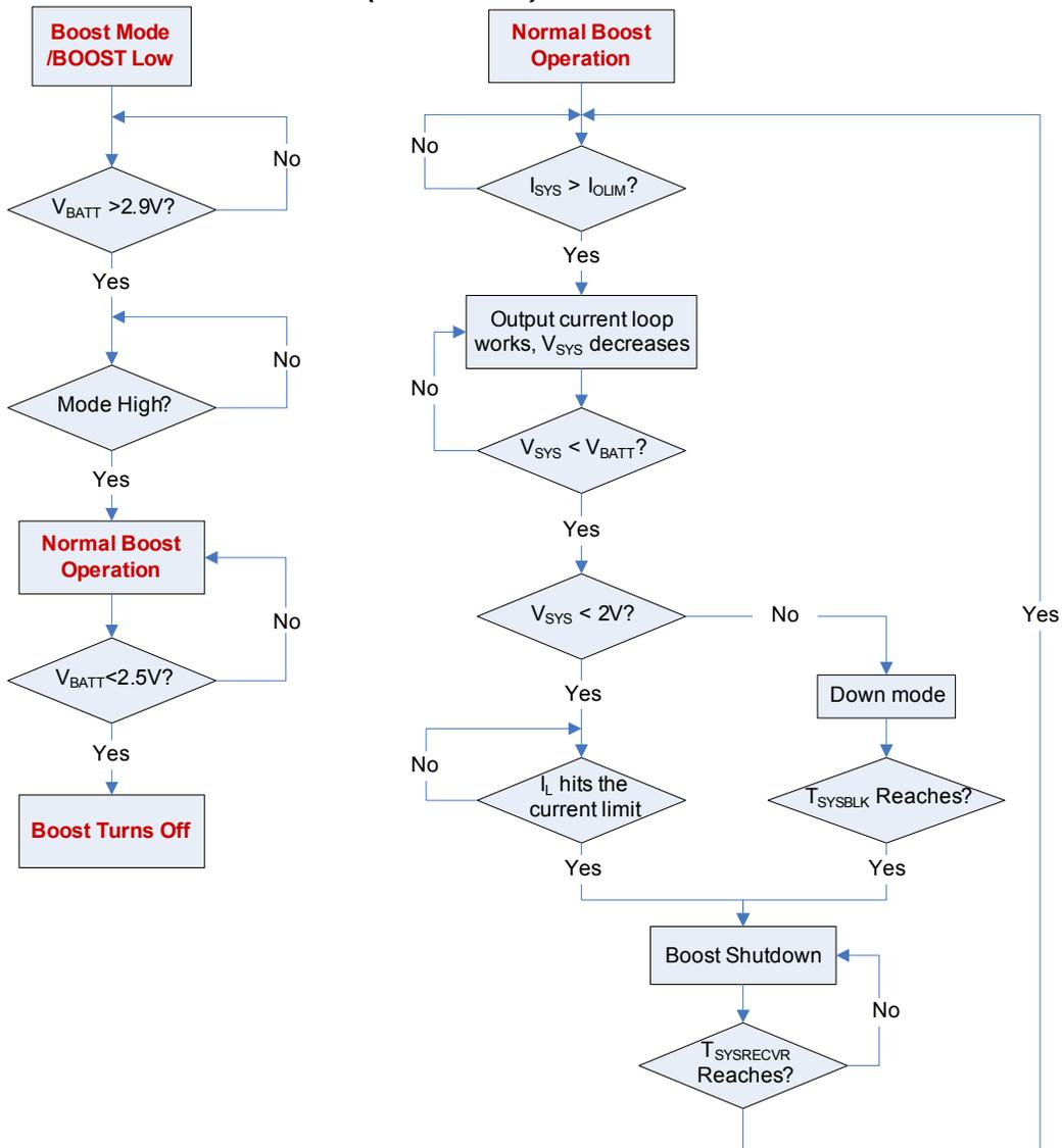
**Figure 6: Operation Flow Chart in Boost Mode**
