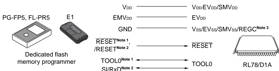
Figure 29-2. Communication with Dedicated Flash Memory Programmer
