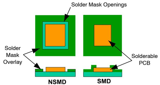
**Figure 8. Comparison of NSMD vs. SMD Pads**
