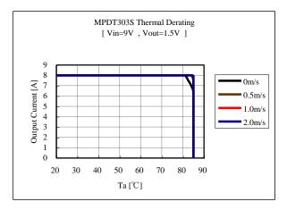
The above derating limits apply to this product soldered directly to 101.6×180mm×1.6mm PCB (double-sided, with 70um copper). Any adjacent parts of high temperature or difference of PCB design may cause overheat of this product. For reliable operation, please check that the FETs temperature of this product is below 120 °C, and the inductor temperature of this product is below 110 °C.
