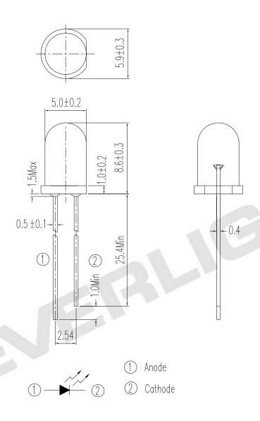
Note: Tolerances unless dimensions ±0.25mm
