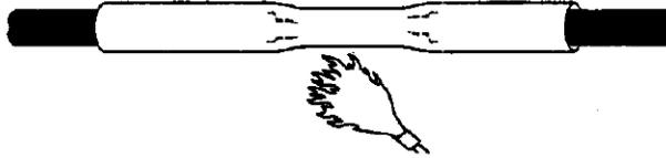
7. Heat until tubing is completely shrunk and adhesive/sealant (if applicable) is squeezed from ends.
