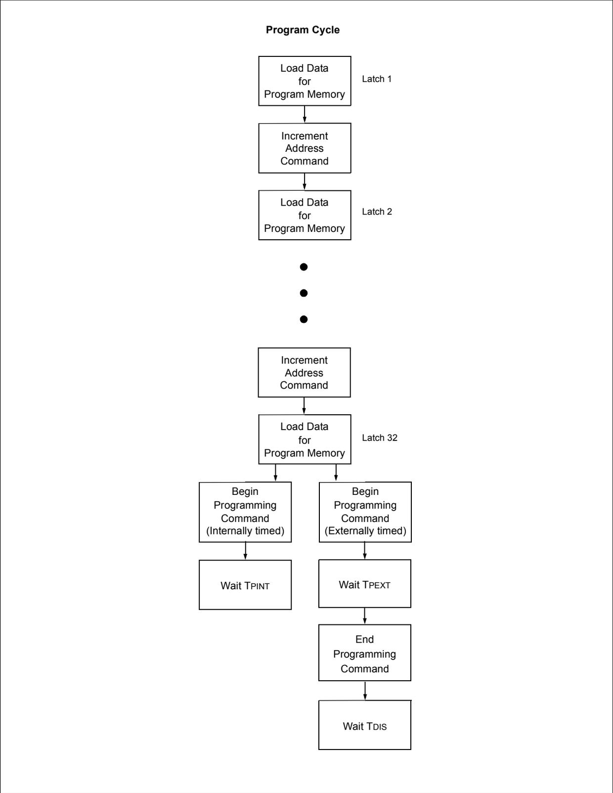
FIGURE 5-5: CONFIGURATION MEMORY PROGRAM FLOWCHART
