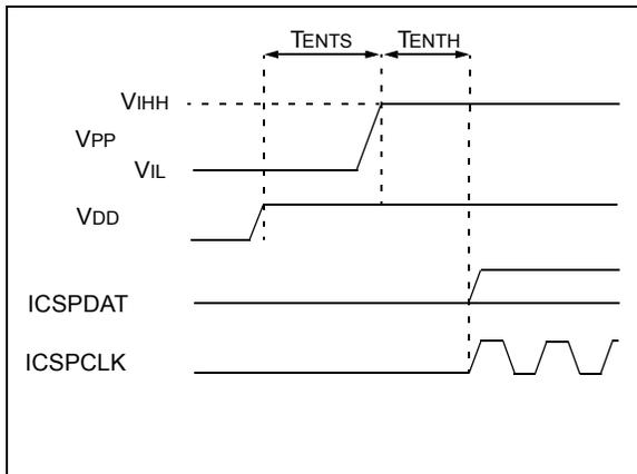
**FIGURE 8-2: PROGRAMMING MODE ENTRY – VPP FIRST**
