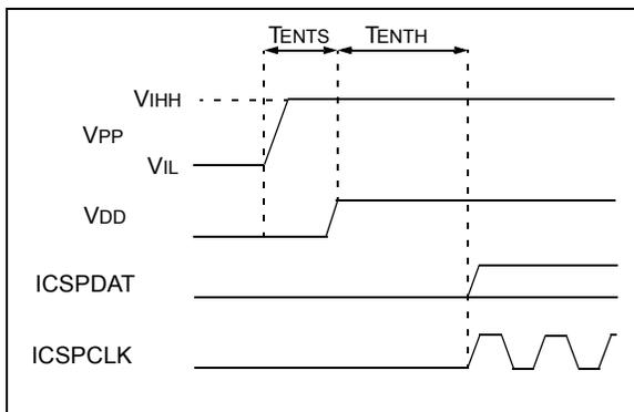
**FIGURE 8-3: PROGRAMMING MODE EXIT – VPP LAST**
