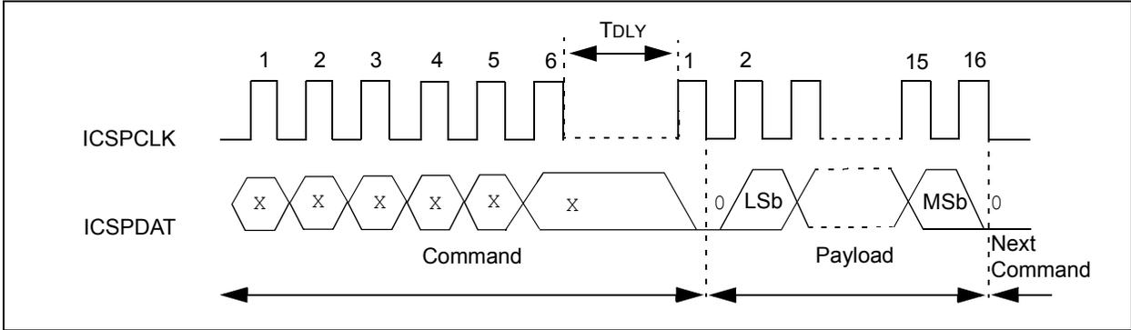
**FIGURE 8-7: READ COMMAND – PAYLOAD TIMING**
