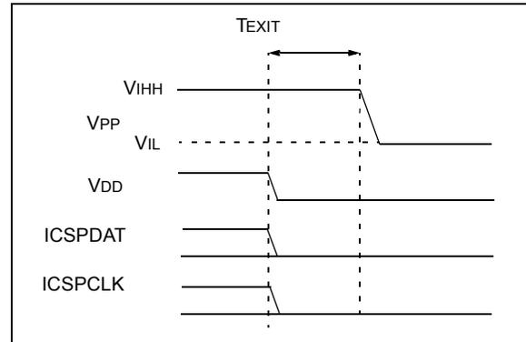
**FIGURE 8-4: PROGRAMMING MODE EXIT – VDD LAST**
