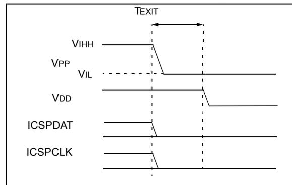
**FIGURE 8-5: CLOCK AND DATA TIMING**
