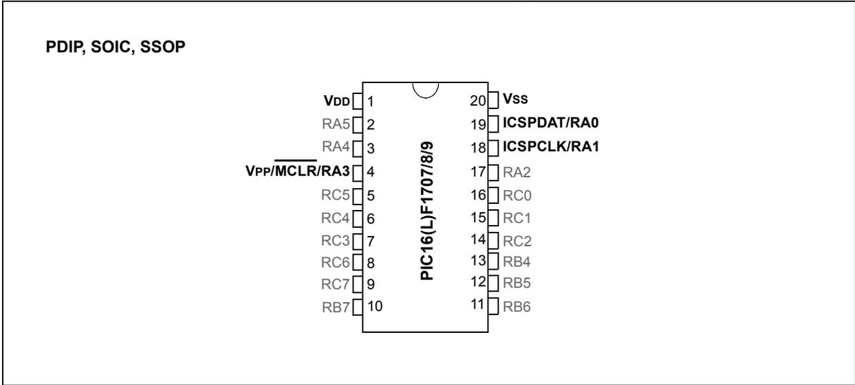
**FIGURE 2-4: 20-PIN PACKAGE DIAGRAM FOR PIC16(L)F1707/8/9**
