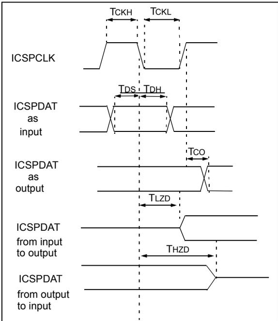
**FIGURE 8-6: WRITE COMMAND – PAYLOAD TIMING**
