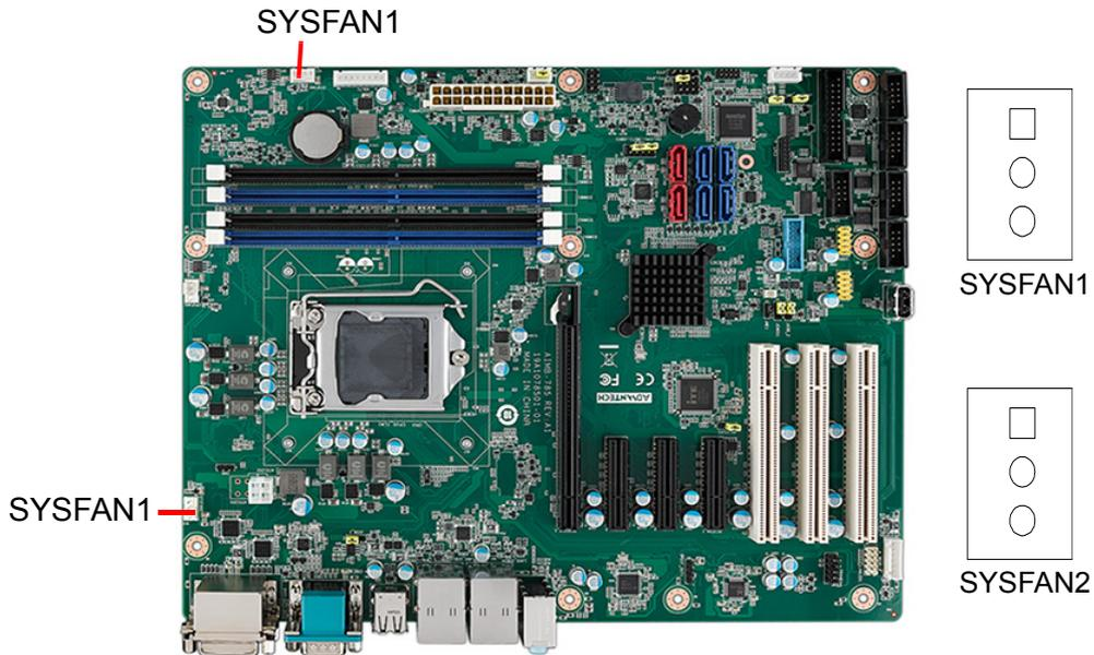
If a fan is used, this connector supports cooling fans that draw up to 500 mA (6 W).
