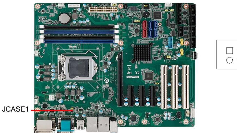
JCASE1 is for chassis with a case open sensor. The buzzer on the motherboard sounds if the case is opened unexpectedly.
