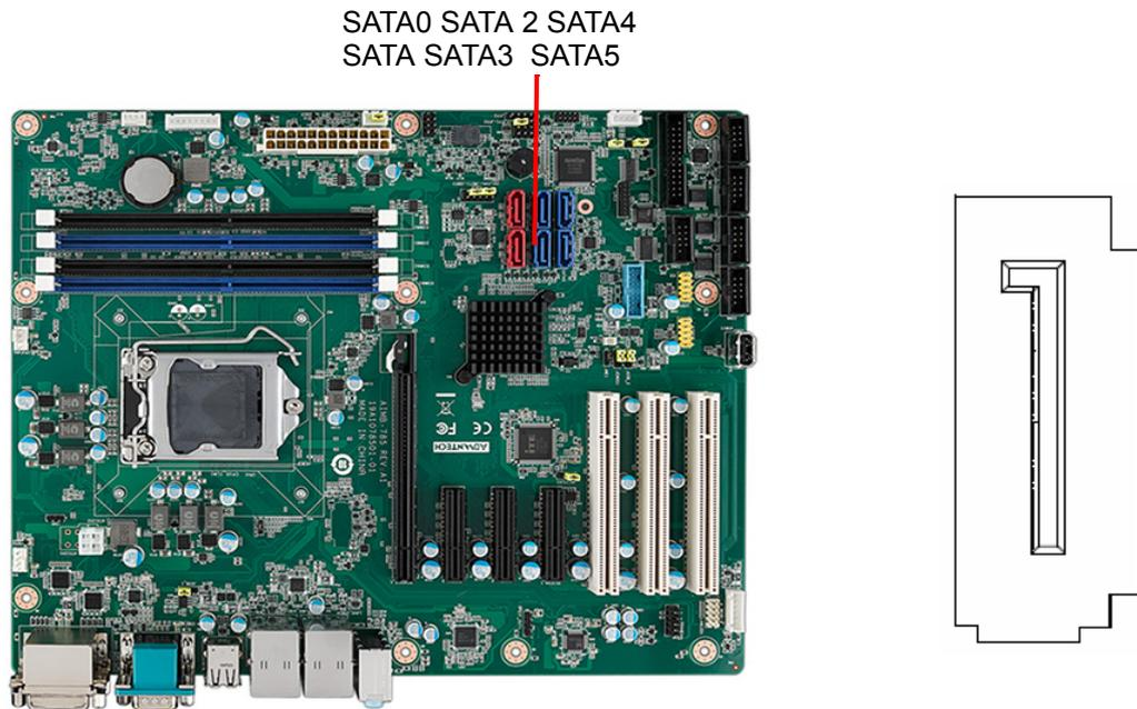
AIMB-785 features six high performance serial ATA III interfaces (up to 600 MB/s) with long, thin, easy-to-run SATA cables.
