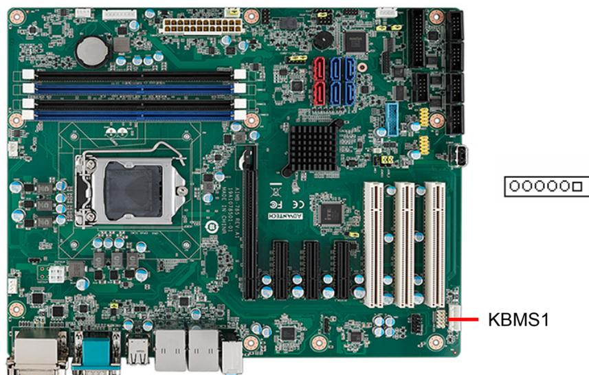
There is also an extra onboard external keyboard and mouse connector on the motherboard. This gives system integrators greater flexibility in designing their systems.
