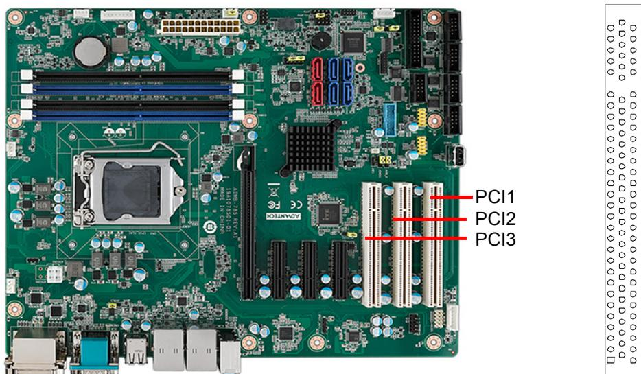
The AIMB-785 provides four 32-bit / 33 MHz PCI slots.
