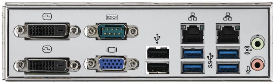
**Figure 1.2 I/O connectors**
