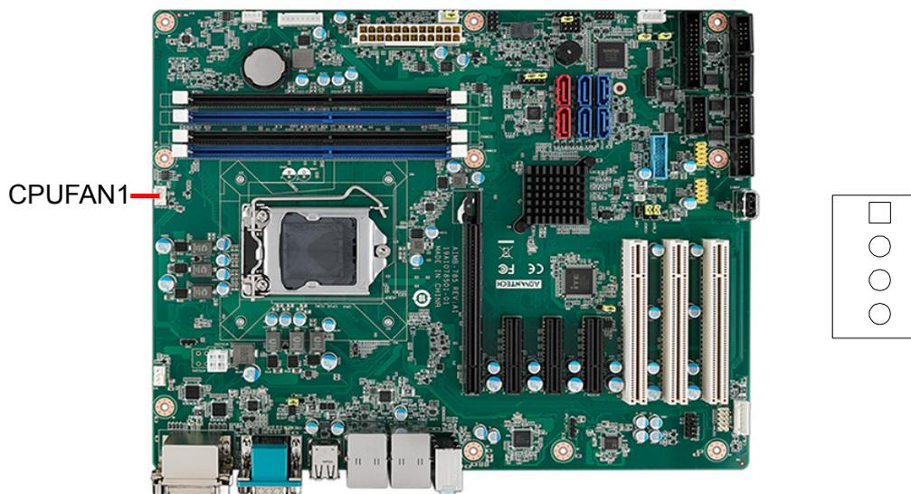
If a fan is used, this connector supports cooling fans that draw up to 500 mA (6 W).
