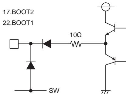
Fig.34 Equivalent circuit
