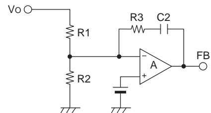
$$\text{Phase lead: } f_z = \frac{1}{2C_2R_3} \text{ [Hz]}$$
