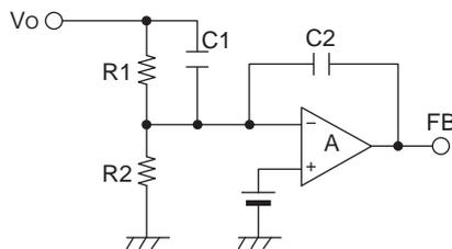
$$\text{Phase lead: } f_z = \frac{1}{2C_1R_1} \text{ [Hz]}$$
