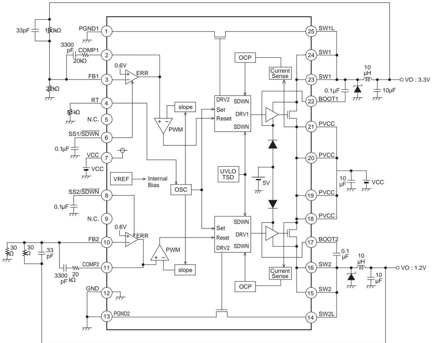
Fig.19 Typical application circuit
