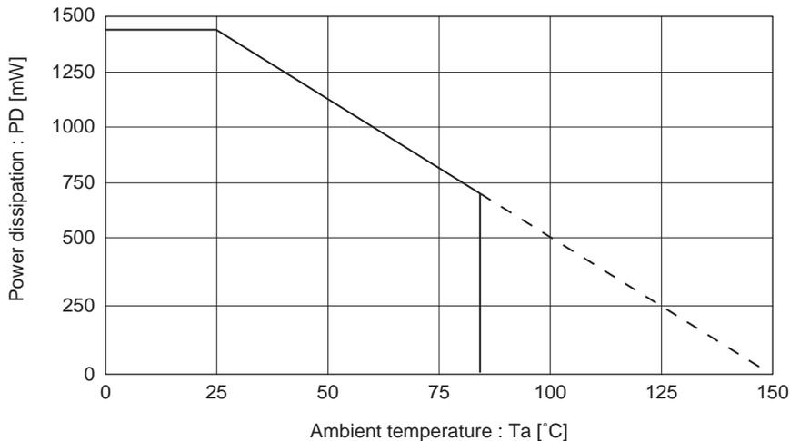
Fig.37 Thermal derating characteristics
