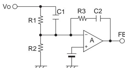
$$\text{Phase lead: } f_{z1} = \frac{1}{2R_1C_1} \text{ [Hz]}$$
