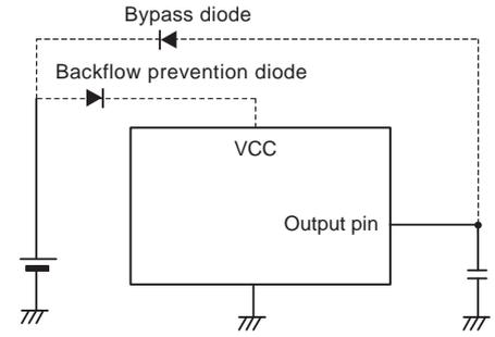
Fig.36 Typical bypass diode application
