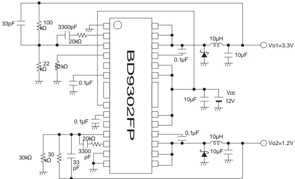
Fig.17 Application measurement circuit diagram
