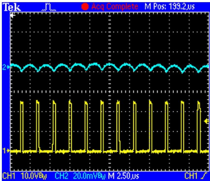
Figure 4. Output ripple at 300mA load.
