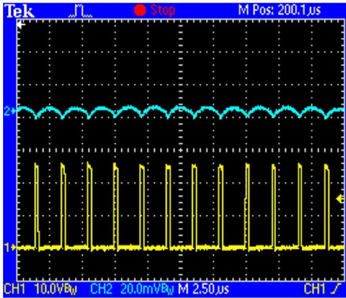
Figure 3. Output ripple at 0mA load.
